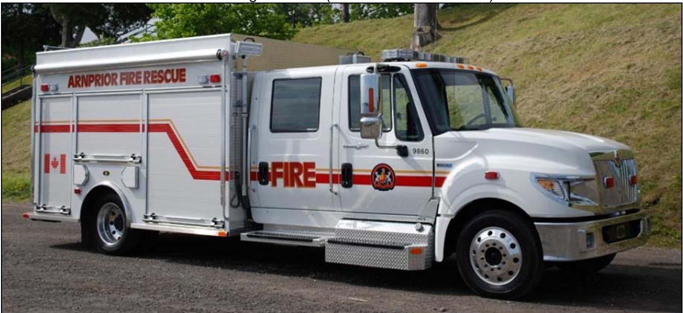
Two not so recent deliveries to Arnprior: Unit 9612, is a 2015 Spartan Metro Star X/Arnprior Fire Trucks rig with a 1050gpm pump and 600gwt. Arnprior 9860 is a 2013 International Terra Star/Arnprior Fire Trucks light rescue. (Photos from Ken Walton)
