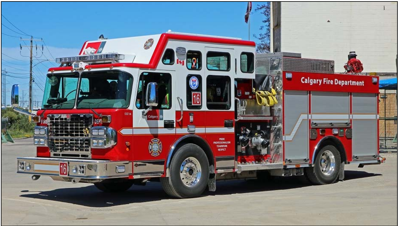
Calgary just received 11 2015 Spartan Gladiator Classic/Smeal 1500igpm(W)/550 gwt/30gft(A)/Eclipse CAFS with Advantus 3 FS (John Bowerman photo). Cummins ISX 500 hp, Allison 4000EVS, 1500 IGPM/550 IG/30AF IG/Eclipse CAFS with Advantus 3 Single Foam System, Single Flush System with off-board pick up, Akron 3440 Deck Master Electric Monitor with Saber Master 1000 IGPM nozzle, Command Light Traffic Flow Board, and Green Power SG-09 Auxiliary Power Unit (Anti Idle Technology), Whelen LED lighting. Learned today that they have ordered another 11 for 2017, and another 5-6 for 2018. (John Bowerman photo)
