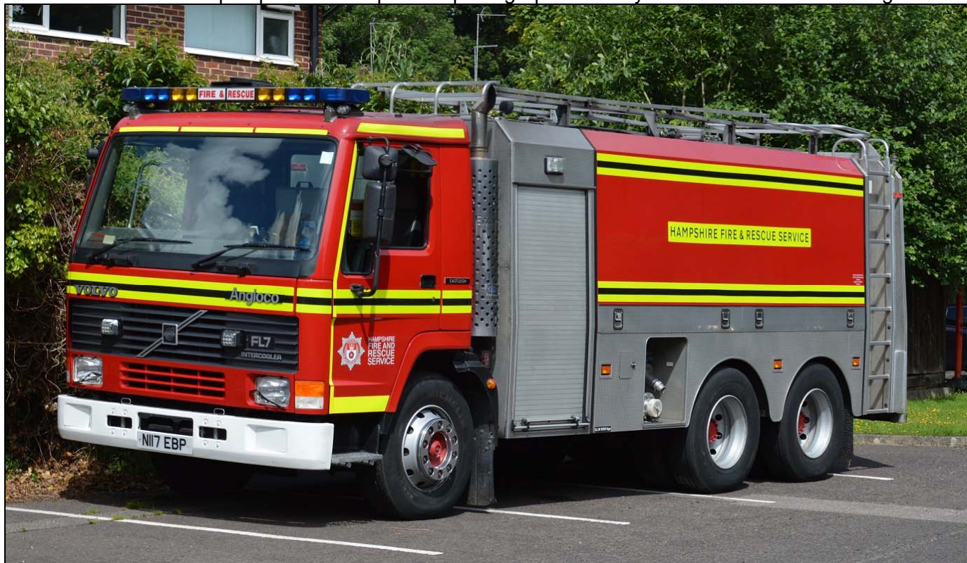
Six Water Carriers are currently in use in Hampshire, two identical to this 1995 Volvo FL7 6x4/Angloco version carrying 10000 litres of water. It is based at Eastleigh and is on the pre-determined attendance for the international airport in the town. (Photos by Colin Carter)
