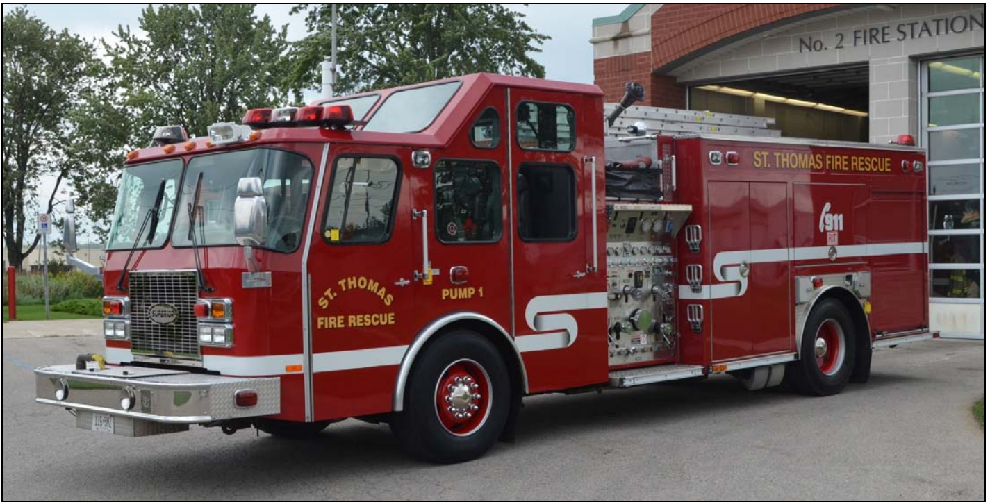
St. Thomas Pump 1, a 2004 E-One Cyclone II / Superior 1750igpm pump & 500gwt. S# 127614, SE 3218
