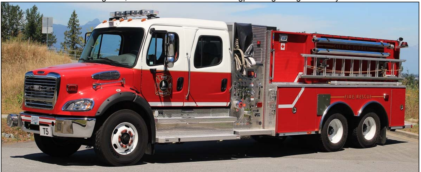
Surrey Tanker 5, a 2015 Freightliner M2-112/Smeal 1500gpm, 2000gwt SO 4379 (Dave Stewardson)
