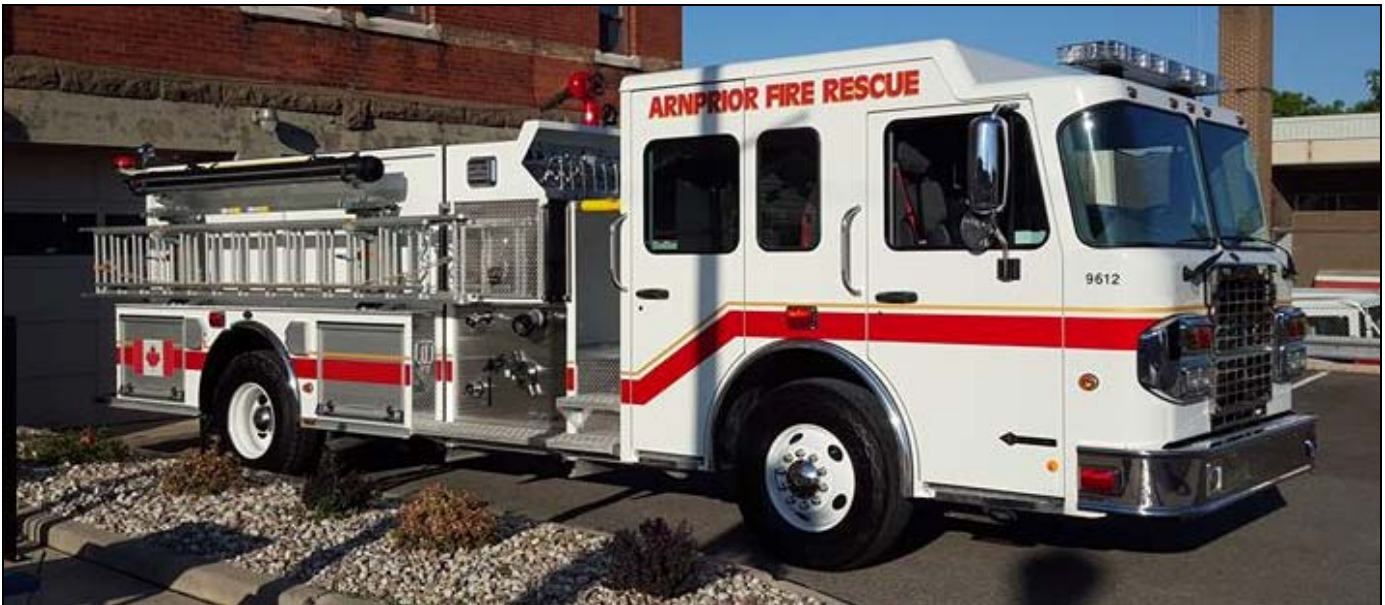
Two not so recent deliveries to Arnprior: Unit 9612, is a 2015 Spartan Metro Star X/Arnprior Fire Trucks rig with a 1050gpm pump and 600gwt. Arnprior 9860 is a 2013 International Terra Star/Arnprior Fire Trucks light rescue. (Photos from Ken Walton)
