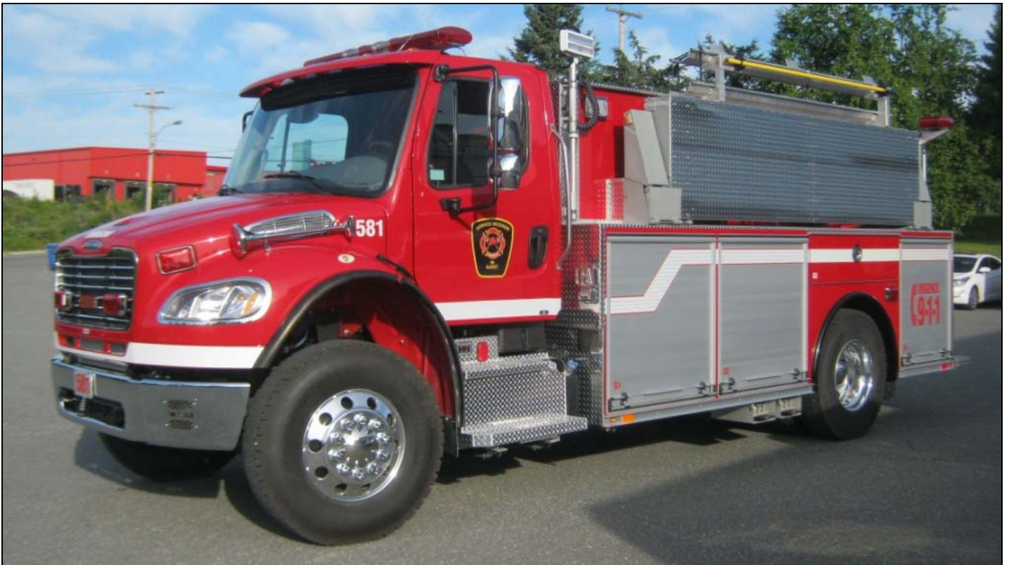
Audet, QC Unité 581 is a 2016 Freightliner M2-106 / Maxi Métal 1500 gallon tanker. (Photo by Maxi Metal Fire Trucks)
