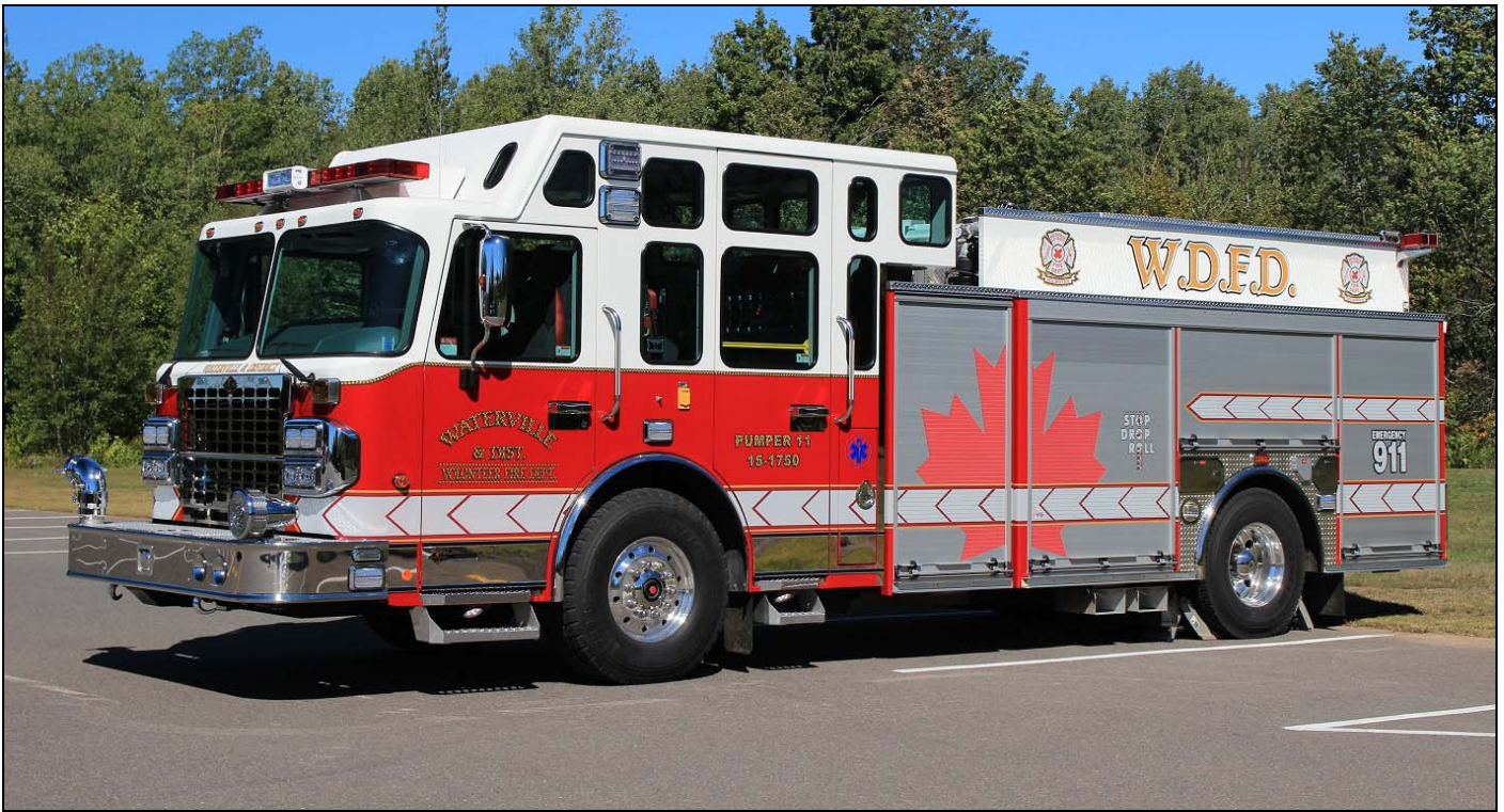
Waterville and District FD in Kings County, Nova Scotia operates from 2 stations. This is Pumper 11 from its HQ's in Cambridge, a 2015 Spartan Metro Star/Lantz rig with a 1750igpm pump, 1000gwt & 25ft.
