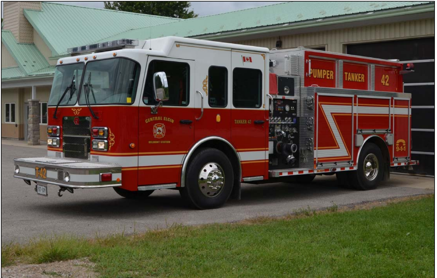
Central Elgin Tanker 42, a 2009 Spartan Metro Star/Rosenbauer/Central, 840igpm/1500gwt. (BobRupert)
