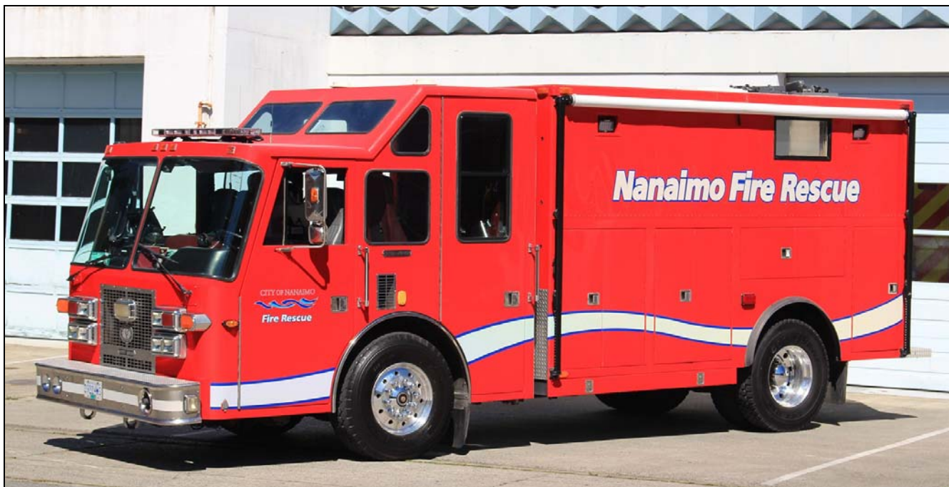
From the B.C. leg of Dave's trip: Logistics 1 is a unit put together by the mechanics at the Nanaimo, BC Fire Dept. The walk-in rescue body came from a 1984 Anderson; the chassis came from a 1992 Simon Duplex pumper also built by Anderson. Body s/n CR-67. (Dave Stewardson photo)
