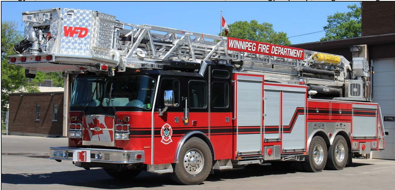
Winnipeg, MB Ladder 1 is a 2016 E-One Cyclone II HP100 tower, featuring a 1750igpm pump and 100' aerial. S/O 139705 (Dave Stewardson photos)
