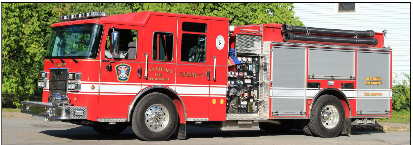
Recently bought by Hantsport in Hants County, NS. E-11 originally served in Arlington County, VA. It responded to the fire at the Pentagon on 9-11. Note the decals that are retained on the rig to mark this event. It also sports a roto-ray. It's a 2002 E-1 Cyclone II 1250igpm/800gwt/20gft(A). SN 124917 (Info and photos from Dave Stewardson)
