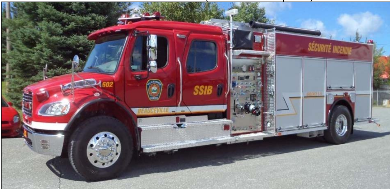
Beauceville, QC recently took delivery of a 2016 Freightliner M2-106/Maxi Métal pumper. Unité 602 sports a 1050igpm pump, 1500gwt and 40gft with a Foam Pro 2001. (Maxi Metal Fire Trucks photo)
