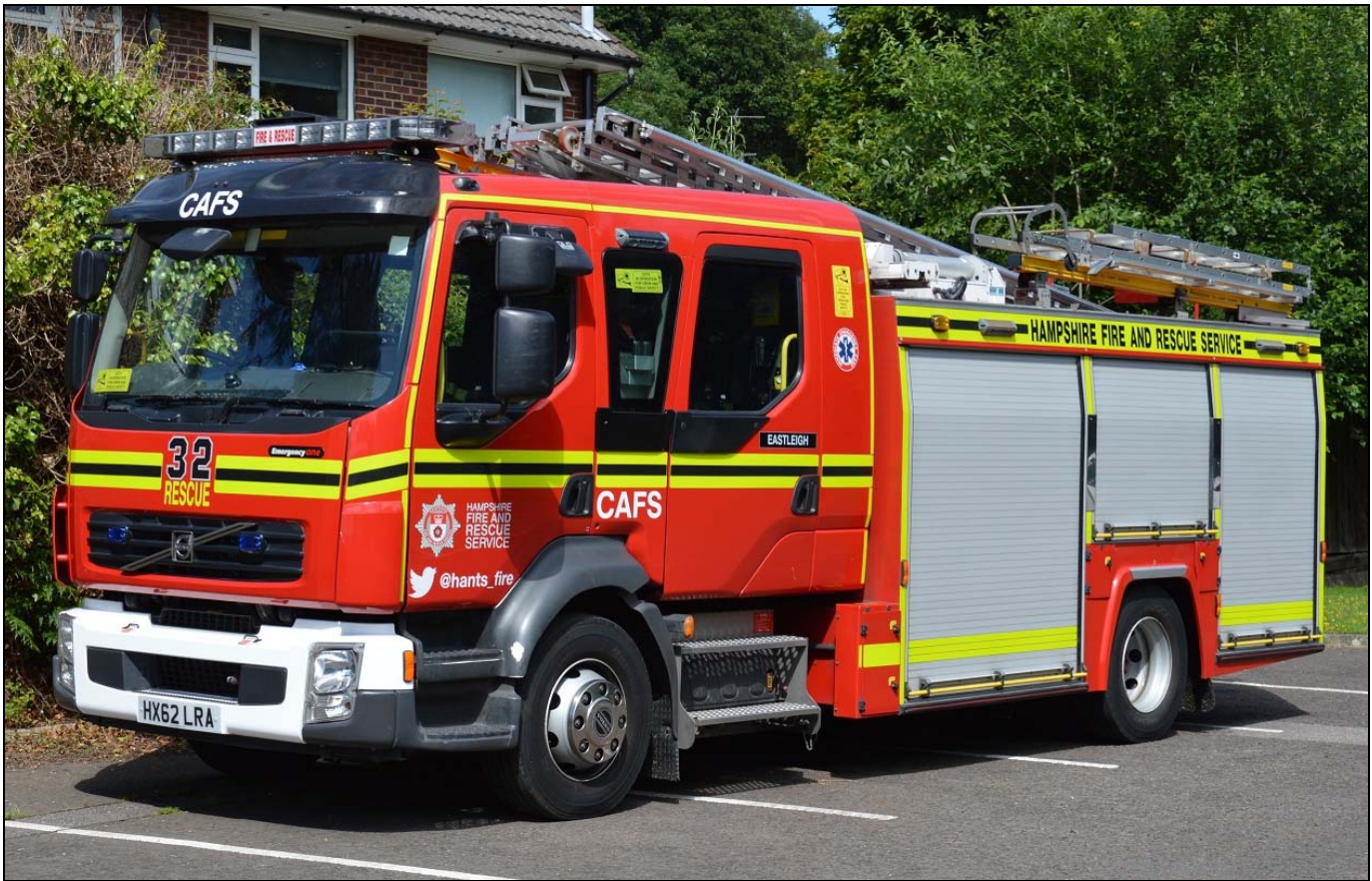
The standard Rescue Pump of which Hampshire currently have 17 is based upon the Volvo FL260 chassis with Emergency One (UK) bodywork. It is equipped with a 1600 litre water tank, 100 litre foam tank and CAFS pump. This example was photographed in July 2016 at station 32 Eastleigh.
