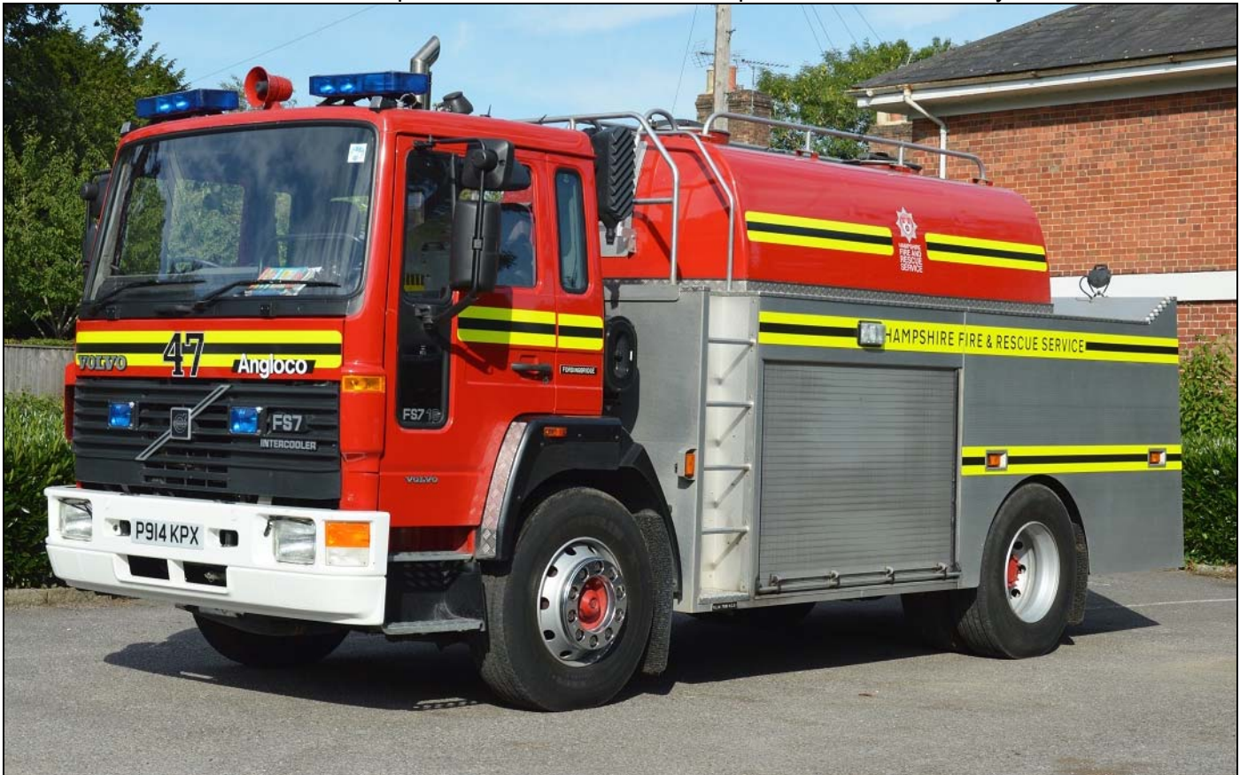
The second type of Water Carrier in the Hampshire fleet is slightly smaller carrying 8000 litres of water based upon either the Volvo FS7 or FL618 chassis with bodywork by Angloco. This example, the only one based on the FS7 chassis is based at station 47 Fordingbridge. (Photos by Colin Carter)
