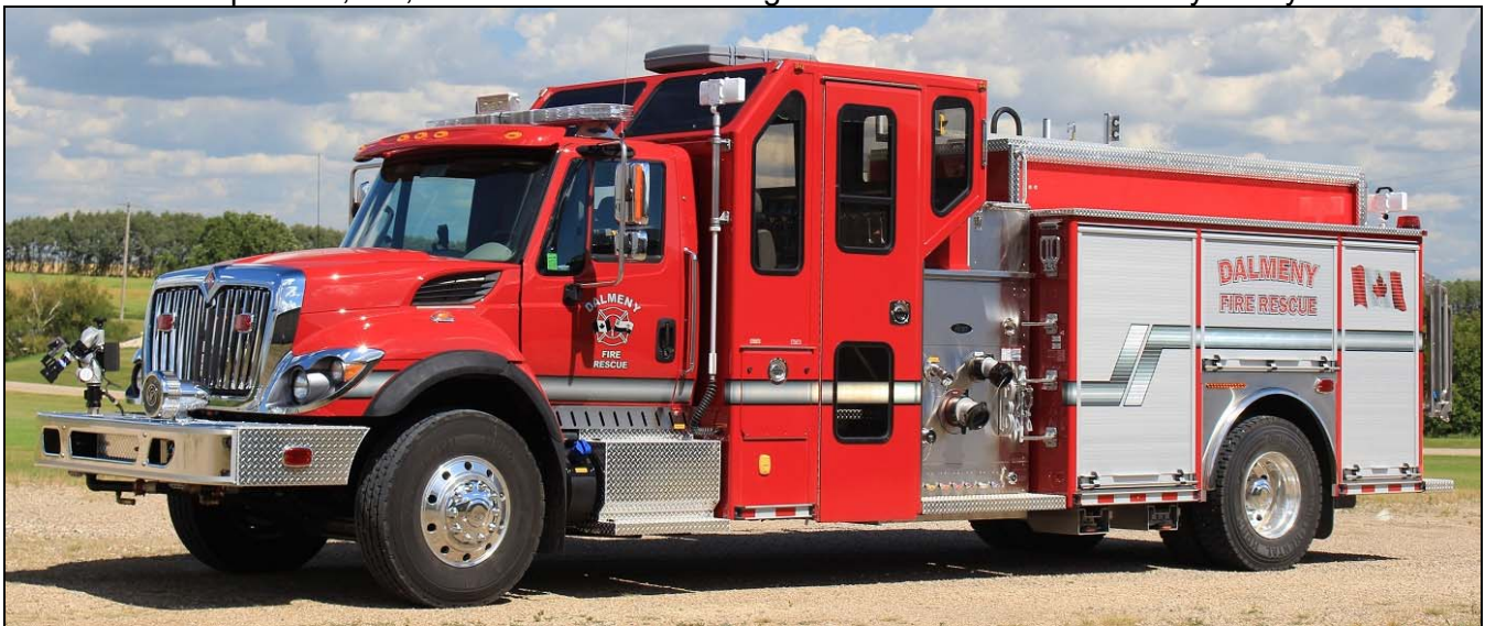
Dalmeny, SK now has this 2016 IHC 7400/Acres pumper. It is equipped with a 1050igpm Hale pump, 1000gwt and 25gft. s/n 1660803143 (Dave Stewardson photos)
