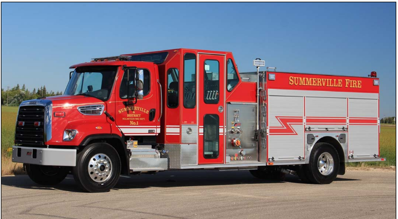
Sommerville, NS recently received this 2016 Freightliner FL108SD/Fort Garry engine. It has a 1250igpm Darley pump, 800gwt, 25gft and Foam Pro 2001. s/n M758. (Dave Stewardson photo)
