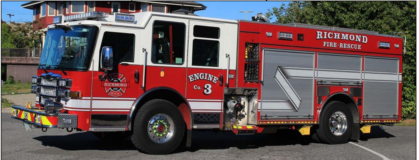
Richmond Engine 3, a 2015 Pierce Dash CF 1500gpm/500gwt/50gft & Husky 12 FS .
