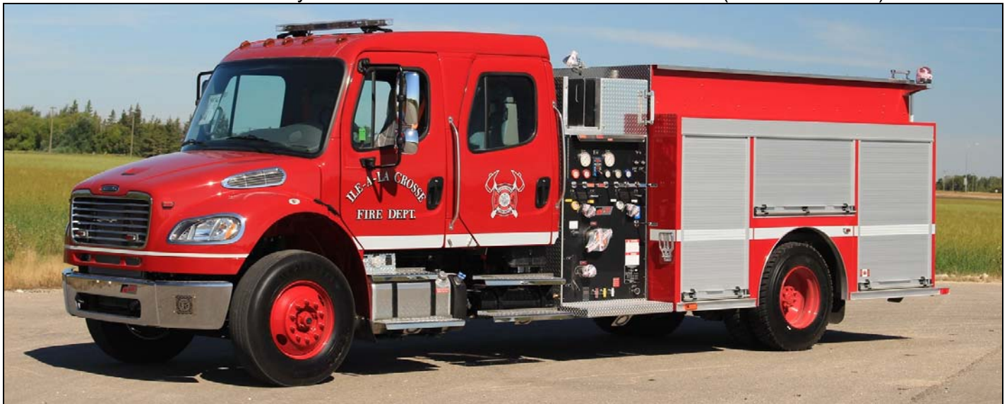
Ile a la Crosse, SK recently got this 2016 Freightliner M2-106/Fort Garry pumper, with a 1050igpm Hale pump and an 800gwt. s/n M743. (Dave Stewardson photo)
