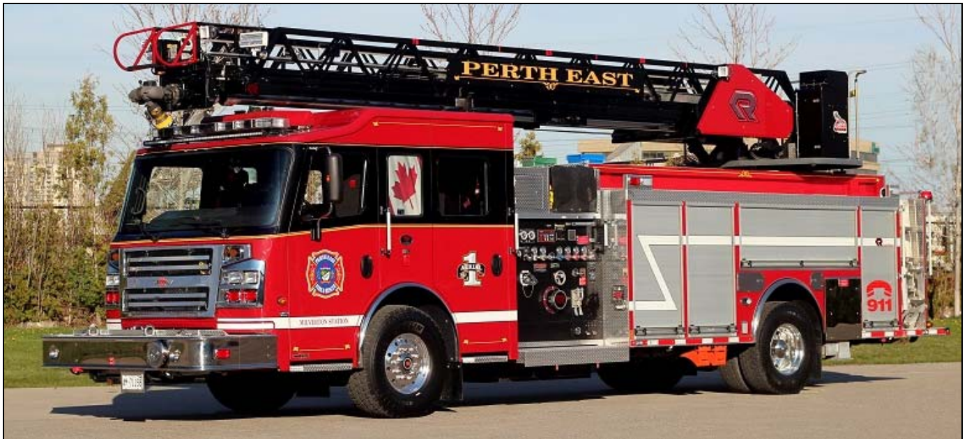
Perth East recently put this 2015 Rosenbauer Commander/Viper 78' quint into service in Milverton as Aerial 1. It features a 1500gmp pump, 400gwt and 60gft (Shane MacKichan photo)
