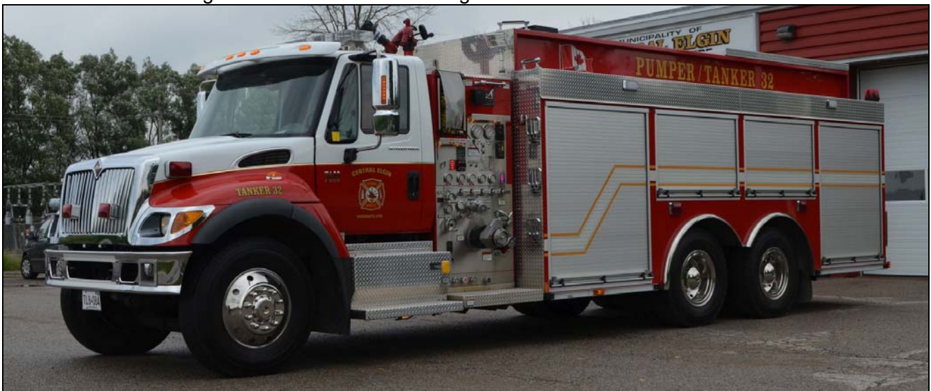
Central Elgin Tanker 32, a 2006 IHC 7400/Smeal, 840igpm pump, 2500gwt and 50gft, S#605070.
