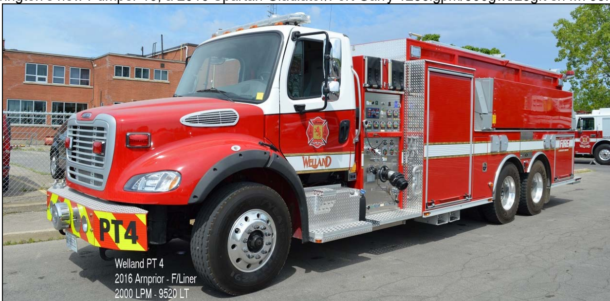
Welland Pumper-Tanker 4 now has a 2016 Freightliner/Arnprior rig with a 440igpm pump and a 2000gwt. Serial #XX6Z5587. (Ken Buchanan photo)
