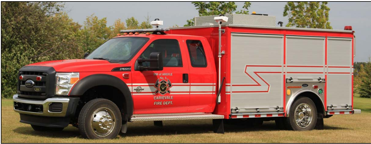
Argyle, SK now has a 2016 Ford F550 4x4/Acres mini, with a 83igpm pump, 400gwt and 25gft.
