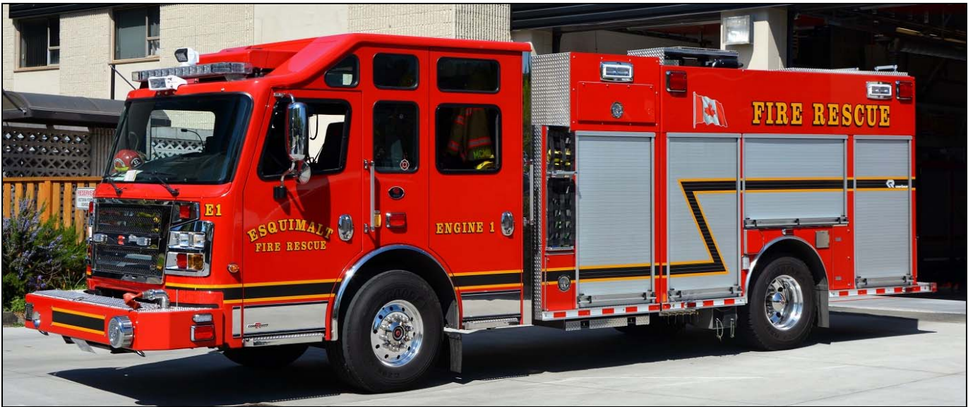
Esquimalt, BC Engine 1 2015 Rosenbauer Commander, 1758 igpm pump, 540gwt, 50ft. (Terry Yip)
