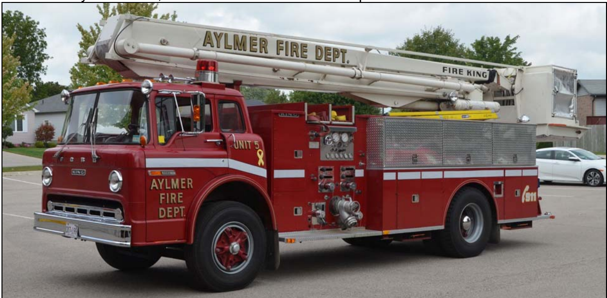
Aylmer Unit 5, a 1978 Ford C900 / King / Snorkel 55' Platform,840igpm, 200gwt. S#77047
