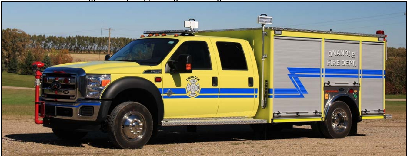
Onanole, MB just received this 2016 Ford F550 4x4/Acres mini-pumper, equipped with a 275igpm Waterous portable pump, 400gwt and 20gft. It has serial number160923146. (Dave Stewardson photos)
