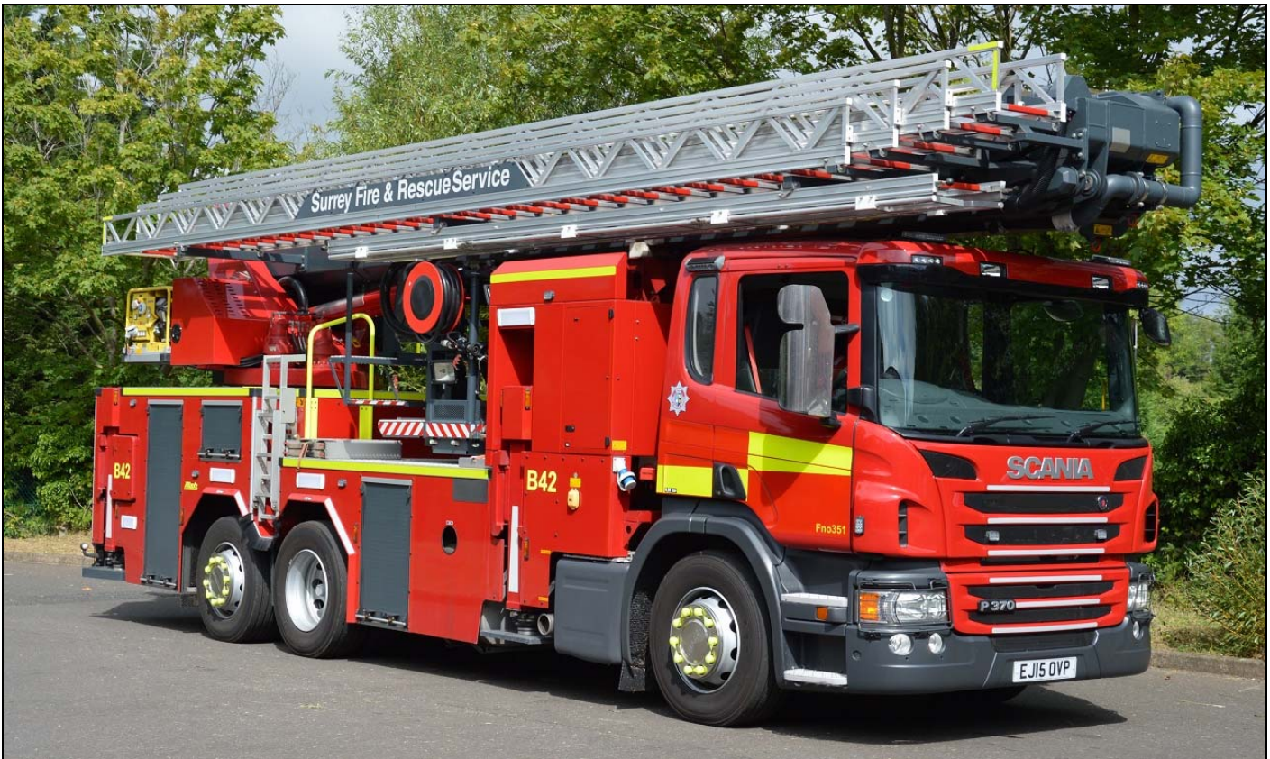
Surrey's 2015 Scania P370/Metz B42 136' Aerial Ladder Platform at Leatherhead Fire Station. This ALP is the only one of its size currently in use in the UK. (Photos supplied by Colin Carter)
