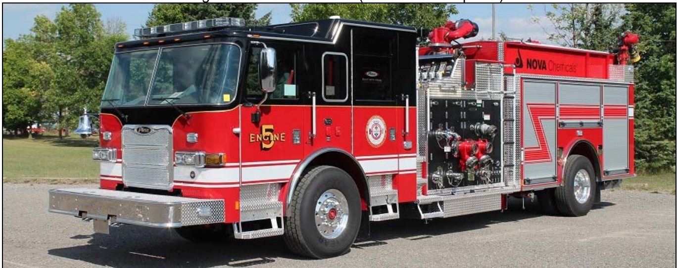
Nova Chemicals (Sarnia) E.5 2016 Pierce Arrow XT 2693 IGPM, 83gft. It has two Elkhart monitors on the rear and one large Akron monitor on the top mid ship. (Gary Dinkel photo)
