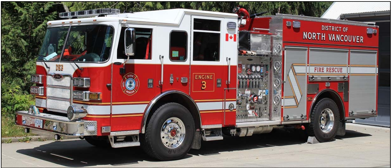
North Vancouver Distrit received a pair of these 2016 Pierce Arrow XT pumpers. They have 1750igpm pumps, 330gwts and 25gfts. Engine 3 above has s/n 28956-1 .
