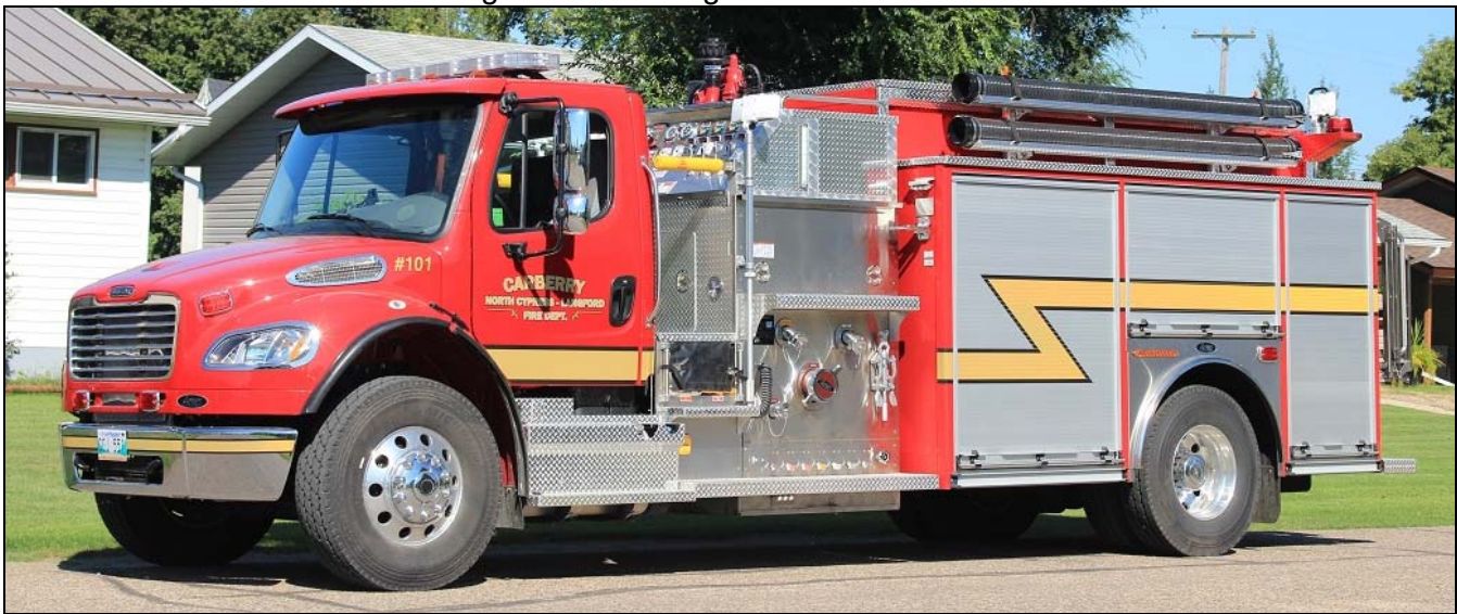
Carberry, MB got this 2016 Freightliner M2-106/Acres pumper for Pump 101 earlier this year. It has a 1050igpmHale pump, 1000gwt and 25gft. Serial number 160610141.
