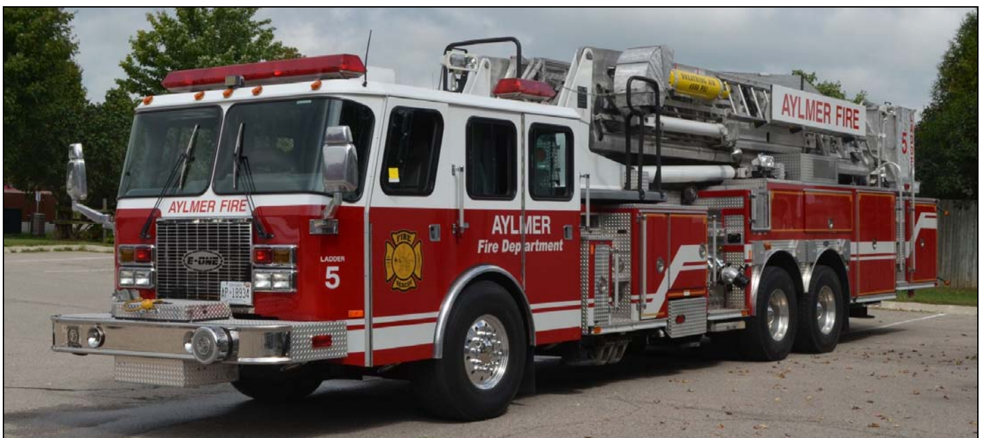
Ladder 5 -2003 E-One Cyclone 95' Platform 1750igpm, 420gwt. S#125919
