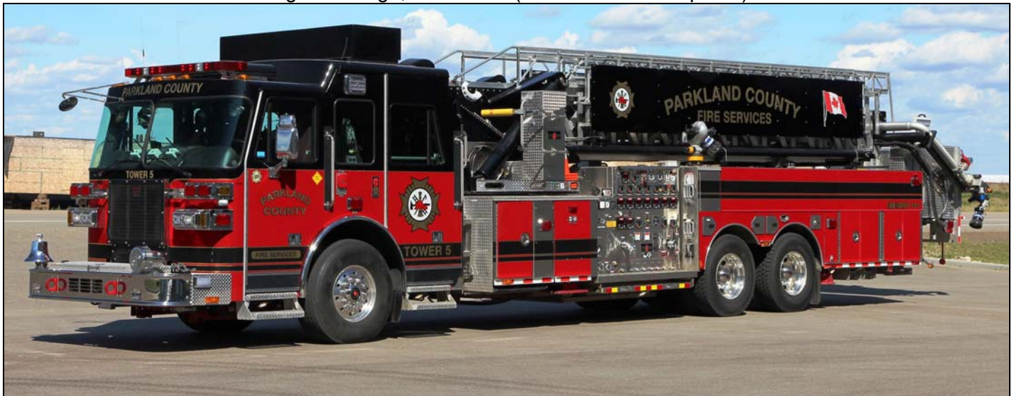
Parkland County, AB bought this 2016 Sutphen Monarch SP112 platform. It has a 112' tower, 3500gpm pump with a FoamPro Accumax 3090 foam system, four TFT Typhoon monitors, a SafetyVision Observer 5 camera system and a mast-mounted TIC in the bucket. (John Bowerman)
