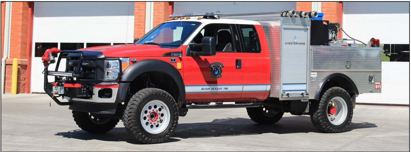
Chestermere, AB Brush Buggy #116 is a 2015 Ford F450 4x4 /Rosenbauer, it has a portable pump, 225gft and 20gft, s/n #3795. (Dave Stewardson photo)
