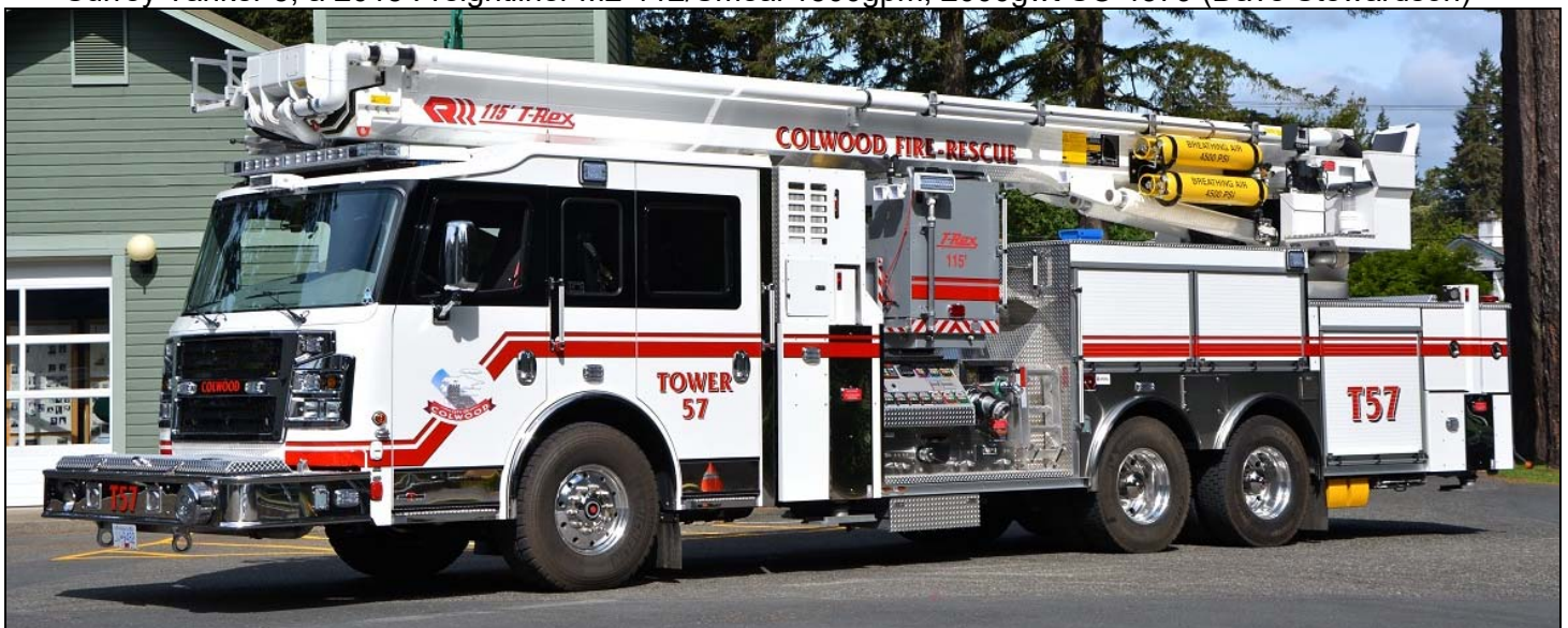
Colwood Tower 57, 2015 Rosenbauer commander/T-Rex 1750igpm/300gwt/115' tower (Terry Yip photo)
