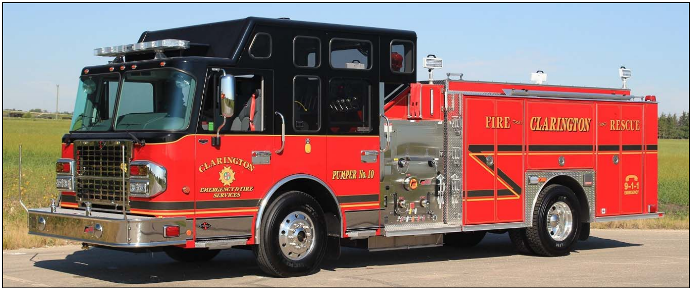
Clarington's new Pumper 10, a 2016 Spartan Gladiator/Fort Garry 1250igpm/500gwt/25gft sn M733.
