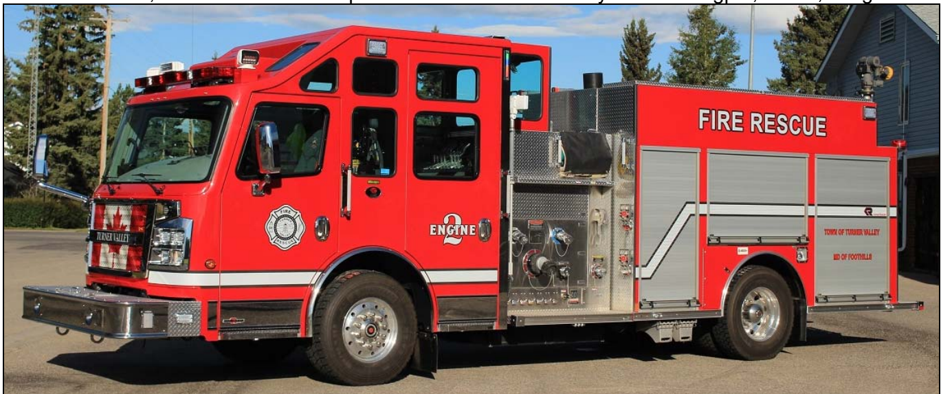
Turner Valley, AB Engine 2 2015 Rosenbauer Commander 1250gpm, 750gwt, 20ft & Foampro 2001 foam system, s/n 16593. (Dave Stewardson photos)
