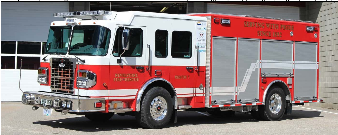
Revelstoke, BC Rescue 7 2015 Spartan Metro Star/Hub heavy rescue 100gpm, CAFS, 300gwt
