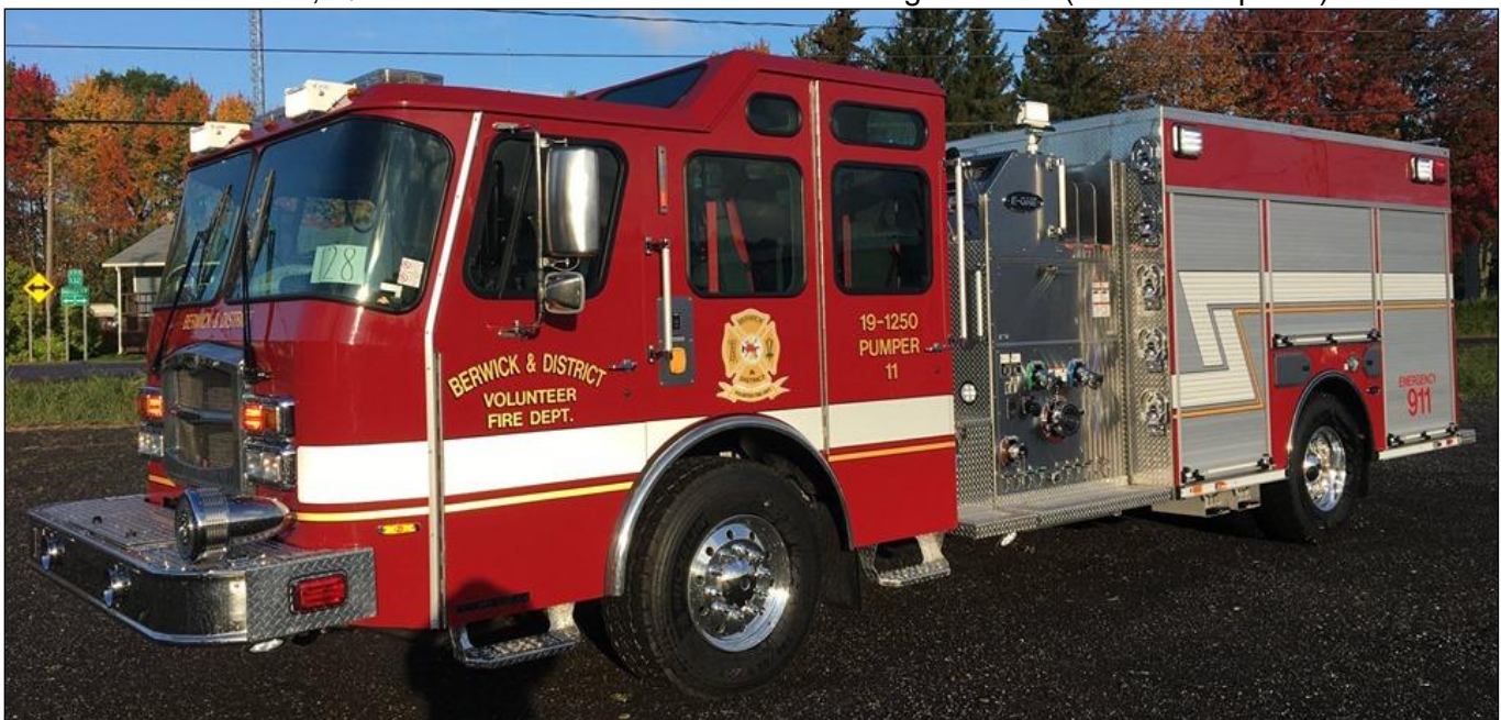
Berwick, NB Pumper 11 - 2019 E-One Typhoon 1250igpm/1030gwt/30gft (SN 142942) (1200 degrees)
