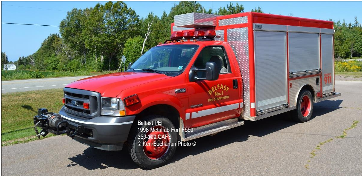
Belfast, PEI Pump 1, a 1998 Ford F550/Metalfab mini with 350igpm pump, 300gwt & CAFS.
