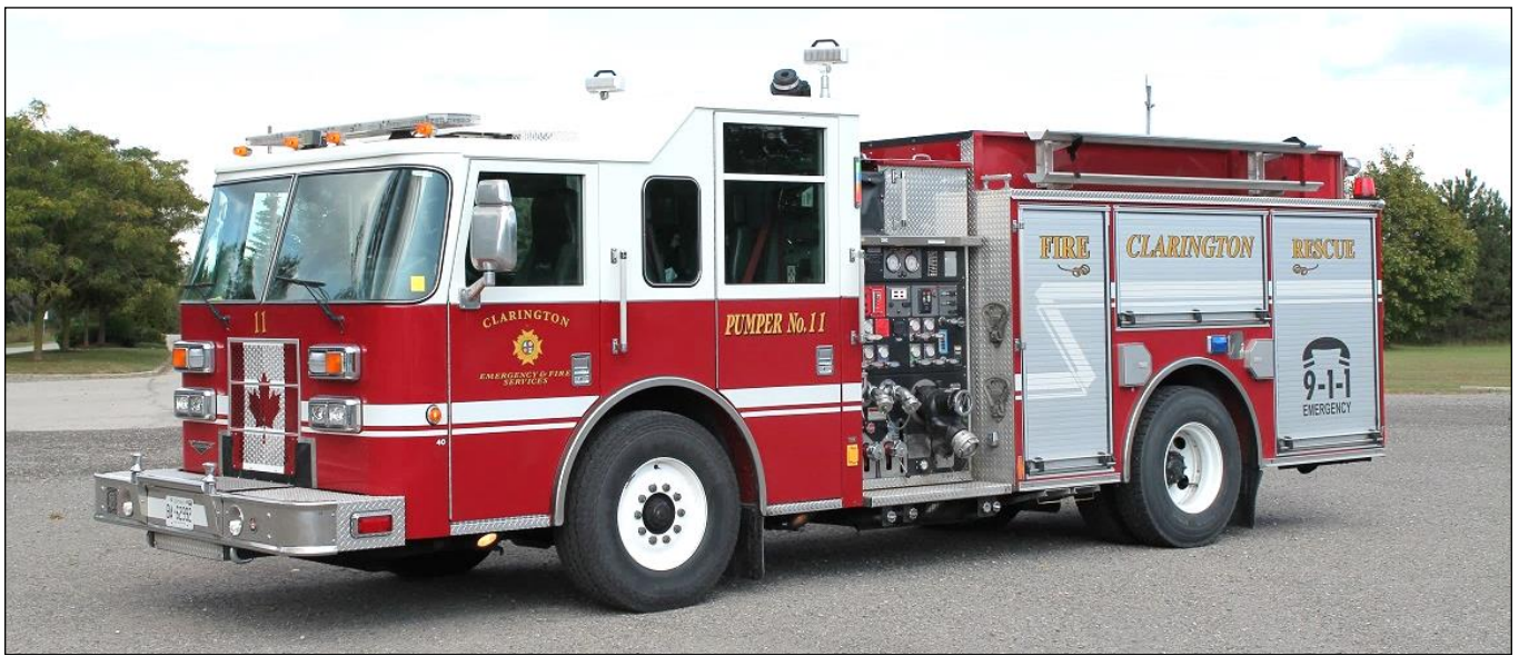
Pumper 11 - 2007 Pierce Saber, 1050igpm pump, 800gwt and 40gft. (SN#19641)
