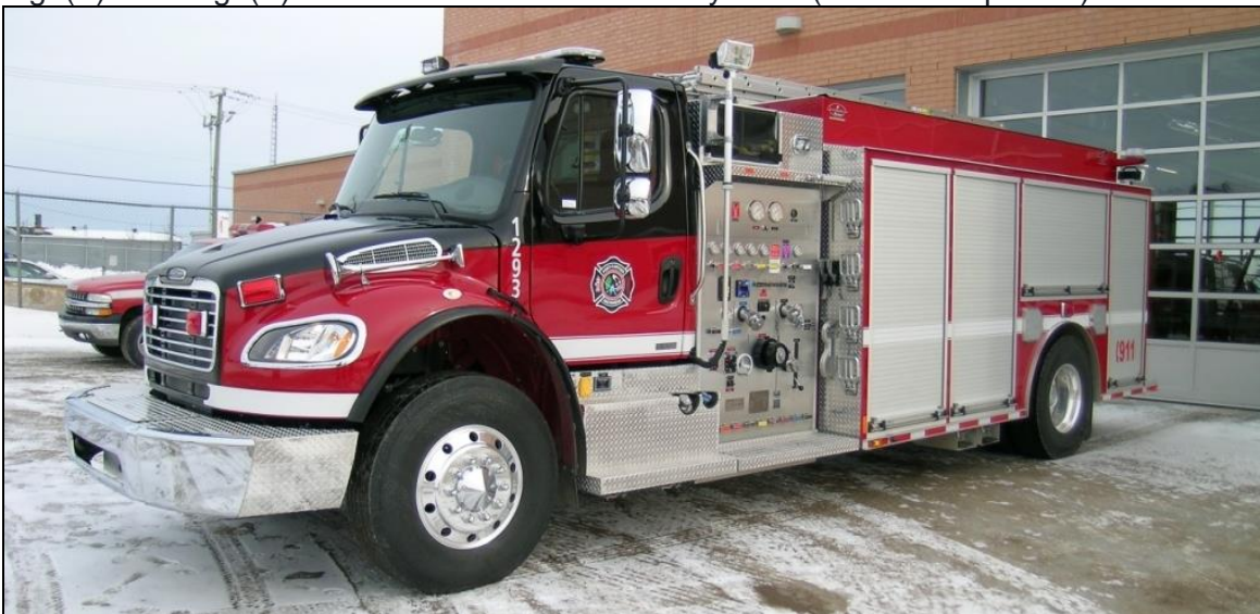
Port Cartier, QC 1293, a 2018 Freightliner M2-106/Maxi Métal pumper equipped with a 1050igpm Hale pump, a 1500gwt and 25gft(A). It also has a FoamPro 2001 foam system.
