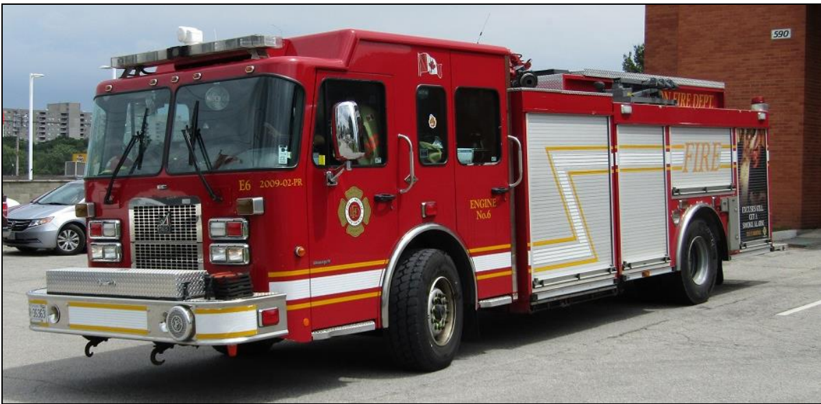
London, ON Engine 6, a 2009 Spartan Advantage/ Smeal rig, 1500igpm/1000gwt/40gft.
