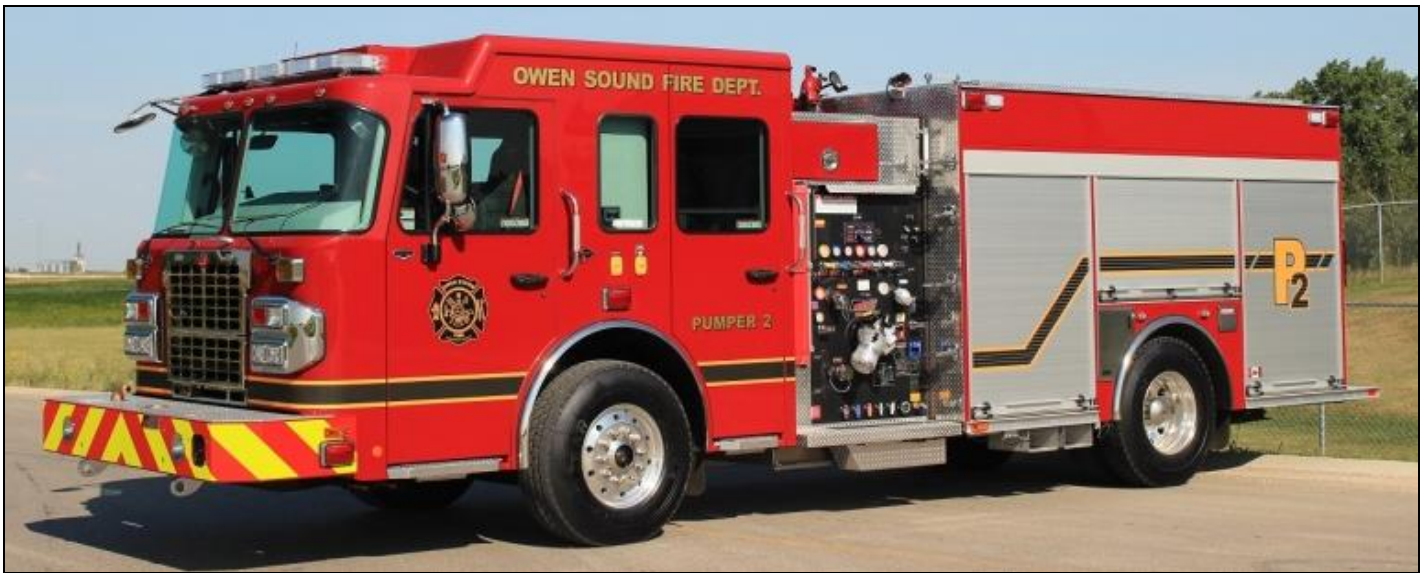
Owen Sound, ON just received this 2018 Spartan Metro Star/Fort Garry pumper, Pumper 2 has a 1250igpm Hall pump, 830gwt and 25gft(A) s/n M880
