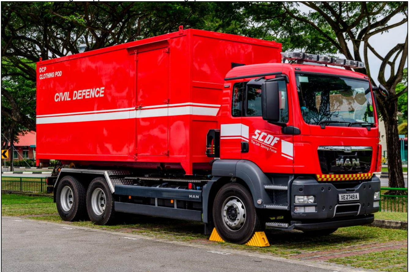
SCDF Pod Carrier, on a MAN chassis. The pod contains clothing for mass decon situations.
