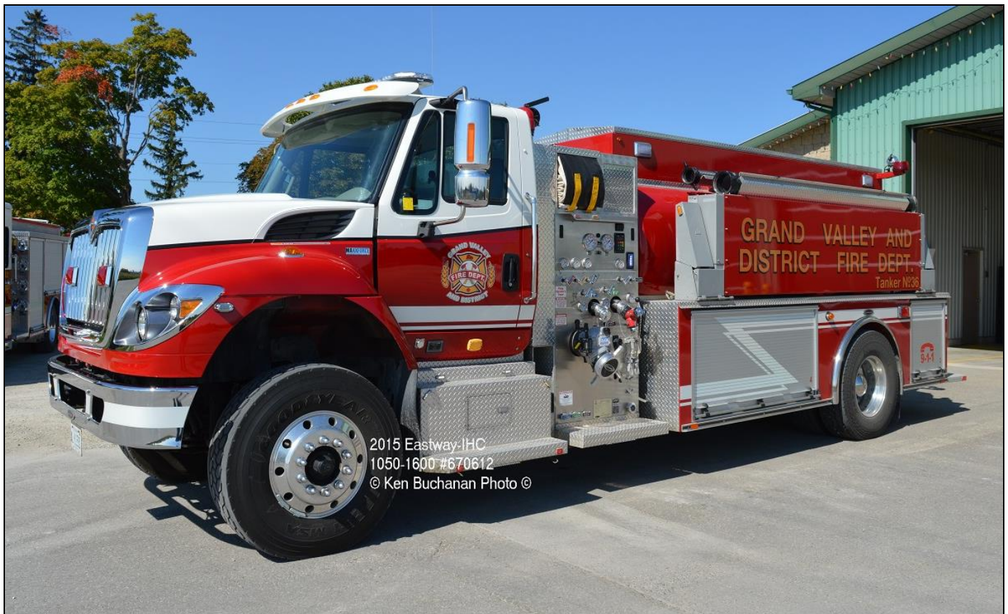
Grand Valley Tanker 36, a 2015 IHC/Eastway pumper tanker, 1050igpm pump and a 1600gwt. SN 670612
