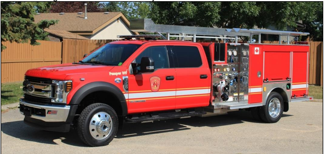
S. Frontenac, ON R.311(R.311 2018 Ford F550/ort Garry 625igpm(D)/300gwt/10gft
