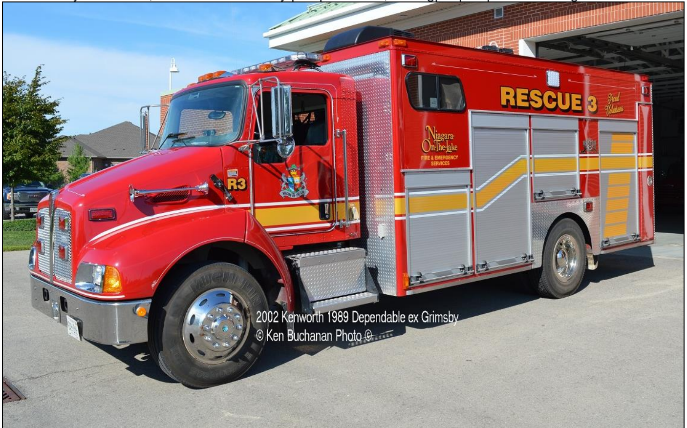
Niagara-on-the-Lake Rescue 3 was completely rehabbed at Dependable with new roll-up doors, new checker plate and, of course, a new paint job. The 1989 DEV box originally belonged to Grimsby and was remounted on a 2002 Kenworth chassis. (Ken Buchanan photos)
