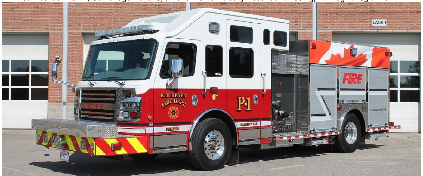
The new Kitchener, ON Pumper 1, a 2018 Rosenbauer Commander R7024 pumper with a 1250igpm pump, 526gwt and a 30gft. Pumper 6 now has a twin to this rig. (Gary Dinkell photos)
