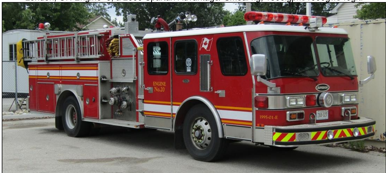
London, ON Engine 20, 1995 E-One Hurricane pumper, 1050igpm/500gwt/40gft.
