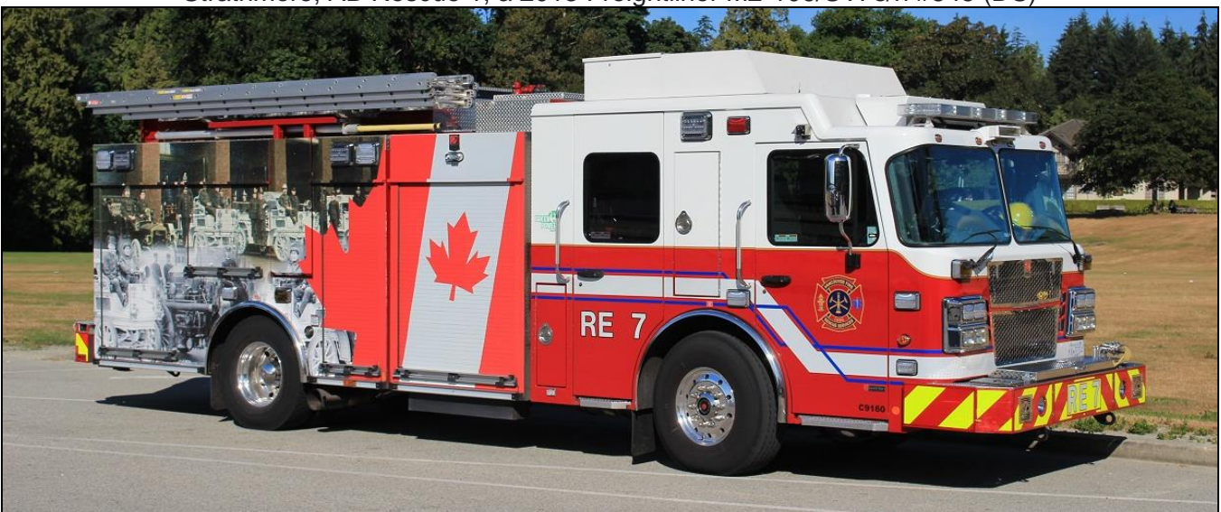
The right side view of Vancouver, BC RE 7 with the Canada 150 wrap. The rig is a 2016 Spartan Sirius/Smeal pumper equipped with a 1766igpm pump, 400gwt, 63gft(A). (Dave Stewardson photos)
