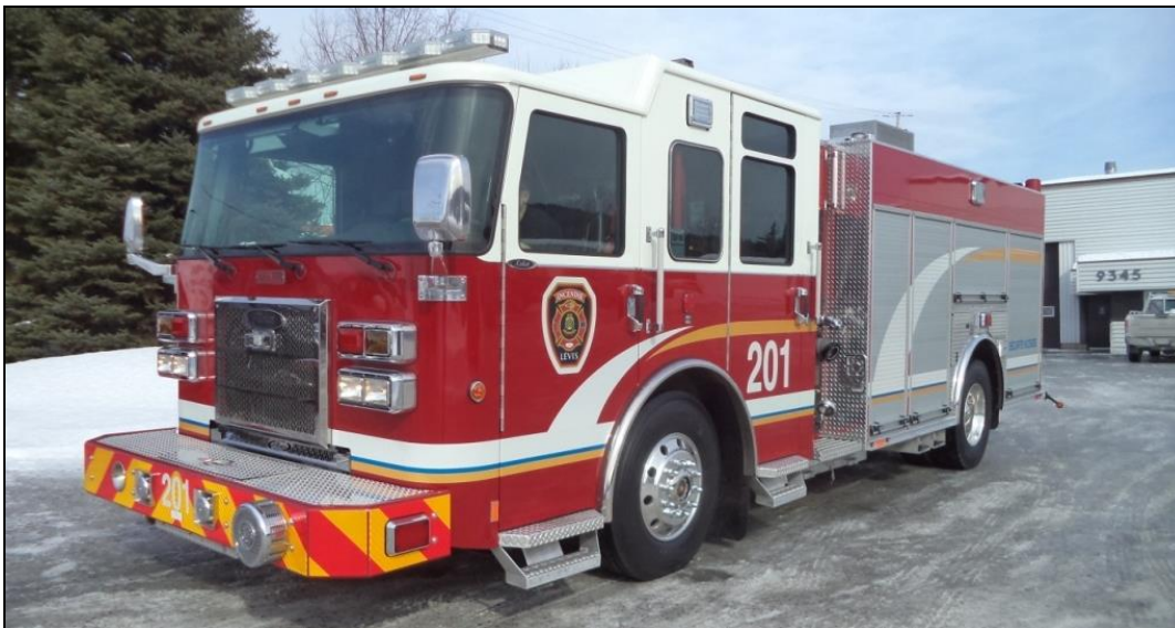
Levis, QC 201, a 2018 Pierce Saber/Maxi Métal engine, 1250igpm Hale pump, 625gwt, 50gft(A) and 30gft(B) with a FoamPro 3012 foam system. (Maxi Métal photos)
