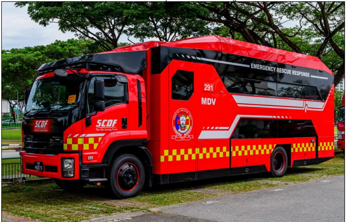
SCDF Mass Decon vehicle was built in 2016 by Hope Technik, a local engineering firm that also designs the Red Rhino light pumps, along with manufacturer Trigen Automotive. It has capacity for eight showers or twelve stretcher patients. (Kenneth Lai photos)
