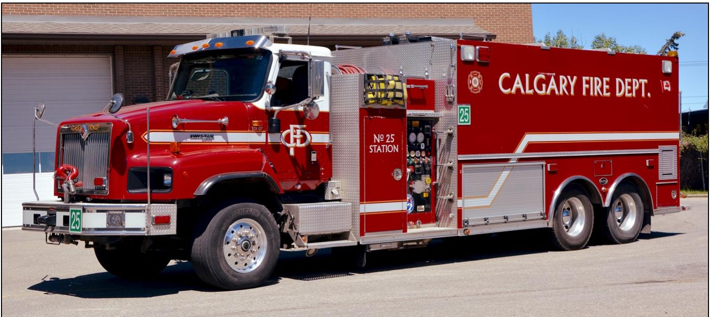
Calgary, AB Tender 25 has a 2007 International Paystar 5000 /Elite rig: 840igpm/3000gwt/10gft(A)/8gft(B).
