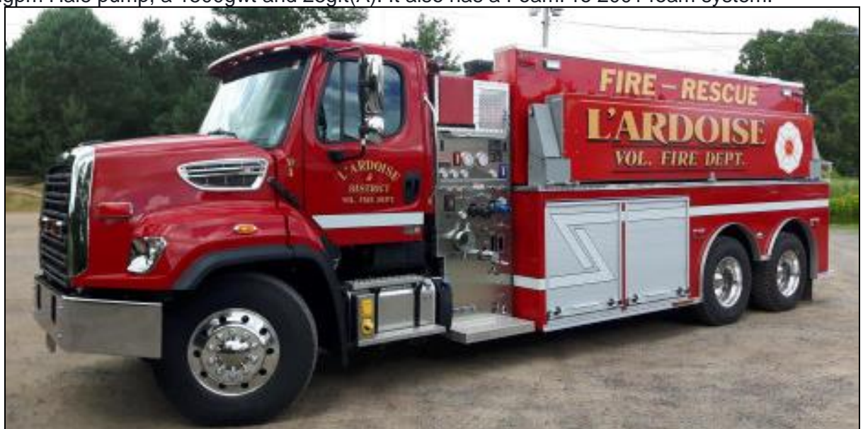
L'Ardoise, NS T.4, a 2018 Freightliner 108SD/Lantz, 1050igpm Hale pump & 3000gwt (Lantz)
