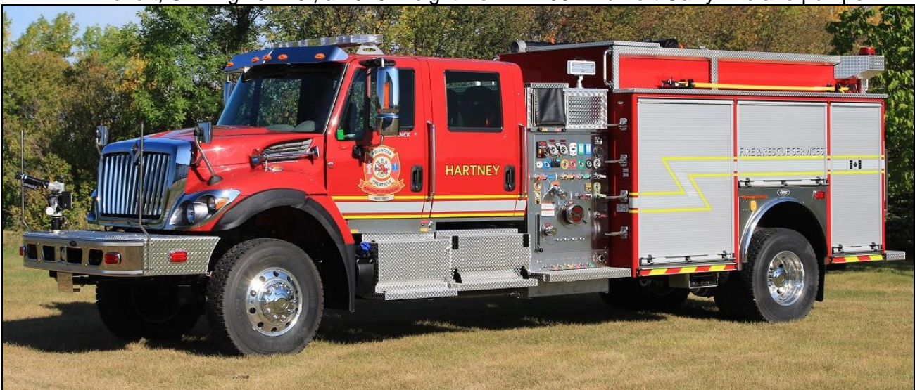
Hartney, MB recently bought this 2018 IHC 7400 4x4 /Acres rural pumper. It has 1050igpm Waterous pump, 1400gwt and 25gft. s/n #180810169.
