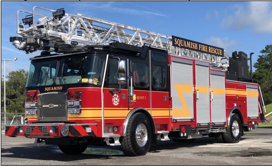
Squamish, BC Quint 2, a 2018 E-One Cyclone II Metro quint, 1500gpm/300gwt/100' SN141764 (E1 photo)
