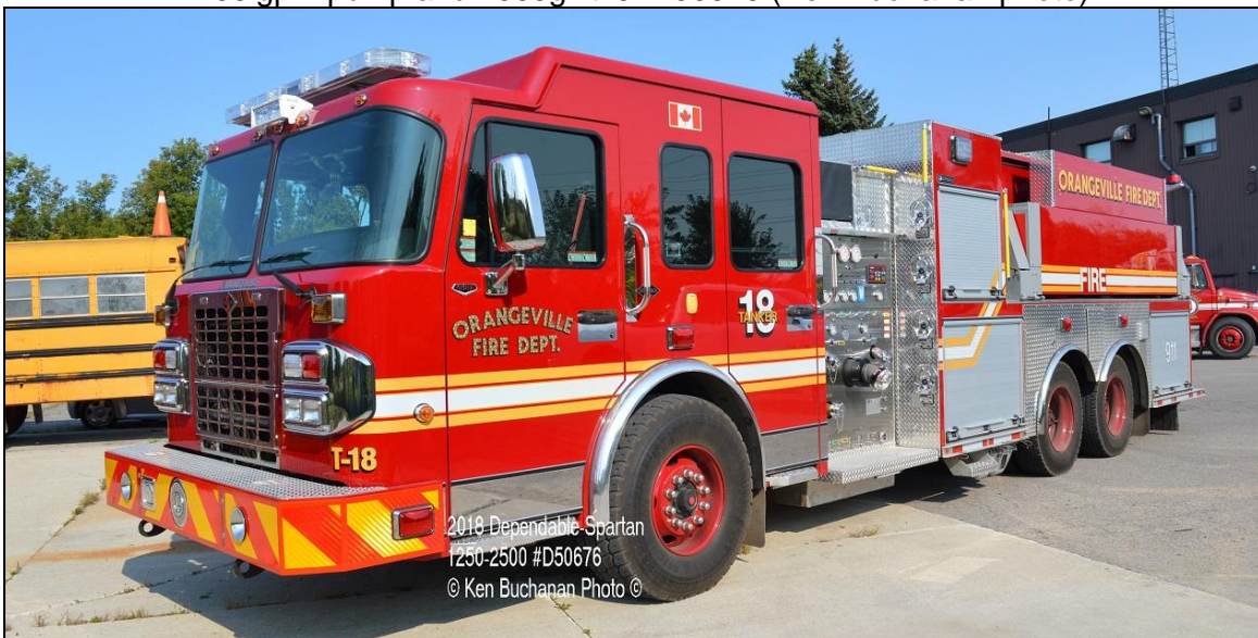
Above: Tecumseh, ON 2018 Spartan Metro Star/Fort Garry 1050igpm/575gpm/25gft s/n M882 (Dave Stewardson photos) Below, Orangeville, ON Tanker 18: 2018 Spartan Metro Star/Dependable with a 1250igpm pump and 2500gwt. J#D50676 (Ken Buchanan photo)
