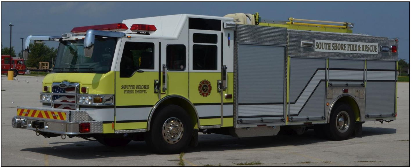
South Shore, WI Engine 9, a 2008 Pierce Velocity rig with a 2000gpm pump and 850gwt, J#19855
