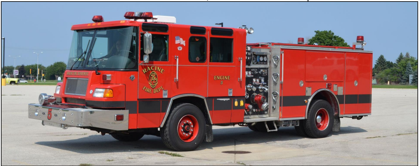
Racine , WI Engine 5, a 2001 Pierce Quantum, 1500gpm pump, 500gwt. J#12639
