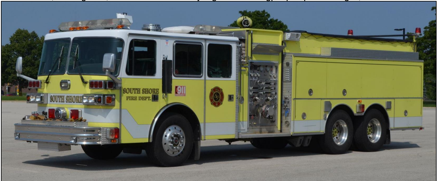
South Shore Engine/Tender 10, a 1994 Sutphen product, 2000gpm pump and 2500gwt, S#HS2871
