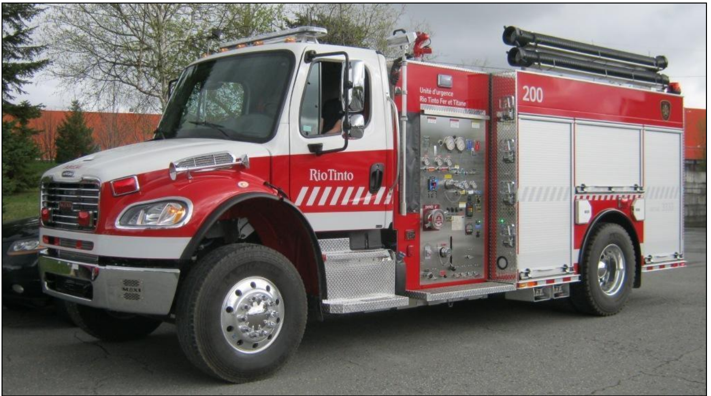
Rio Tinto at Jonquière, QC recently put this 2018 Freightliner M2-106/Maxi Métal pumper-tanker in service. It is equipped with a 1050igpm Hale pump, a 1000gwt and a 40gft(A) Unité 202 also has a FoamPro 2002 foam system.
