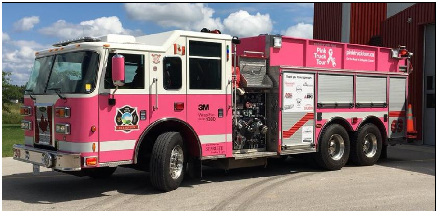
Clearview Tanker 63, a 2013 Pierce Saber wildland pumper tanker, has a 1050igpm pump and 2100gwts. (Photo courtesy Clearview Fire Service)
