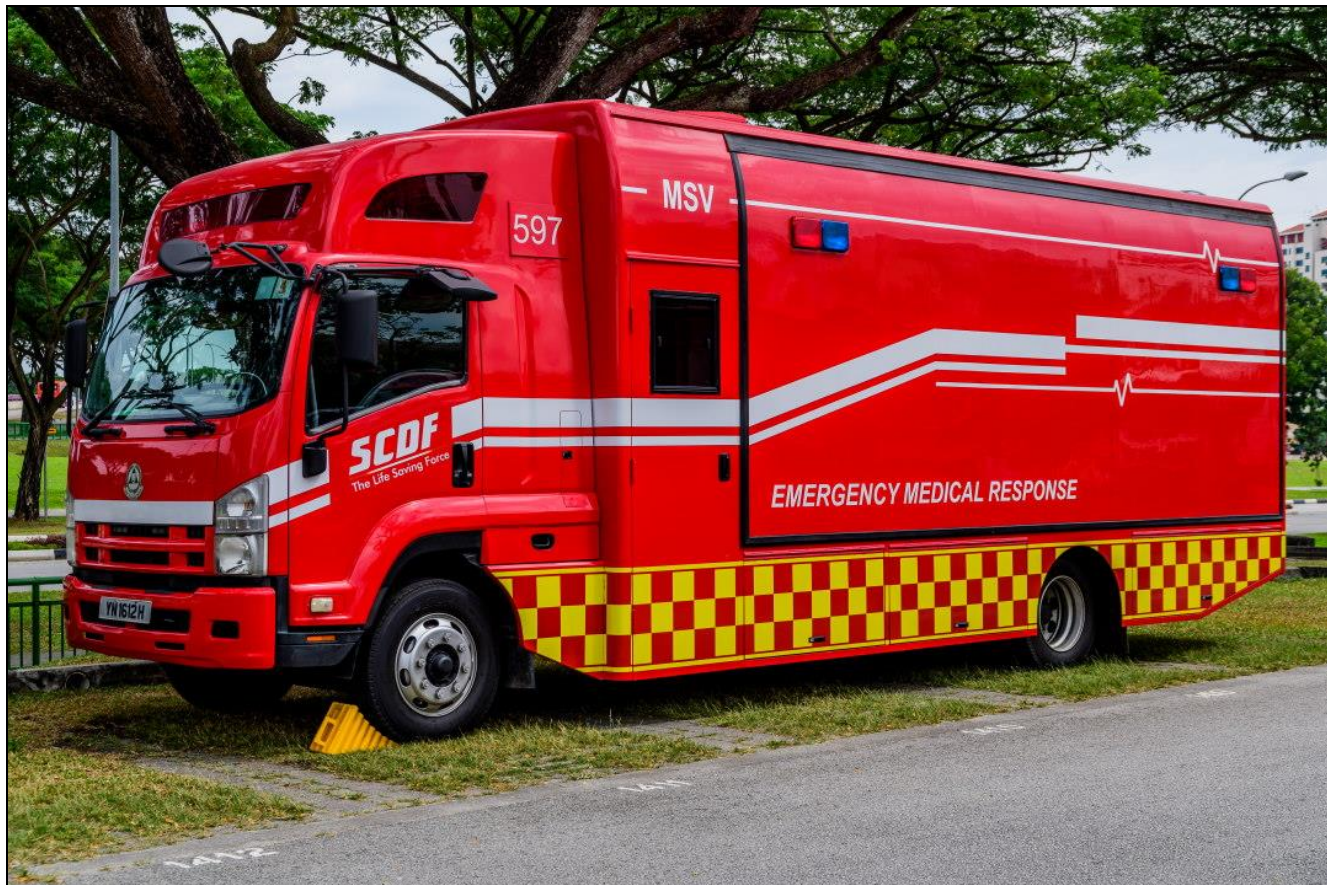
SCDF Unit 597 is a medical mobile treatment unit. Launched in 2013, these units can treat up to eight severe casualties at once. The large panel on the side becomes an awning and allows access to the treatment facilities.
