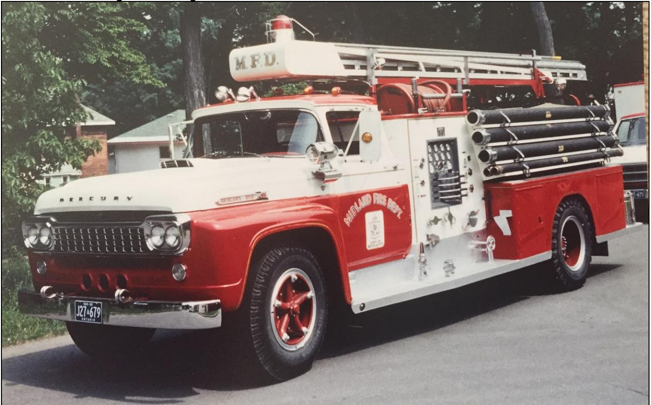
Midland, ON Engine 3, a 1958 Mercury/American Marsh pumper, 625igpm, 500gwt. (Tom Sheppard photo)
