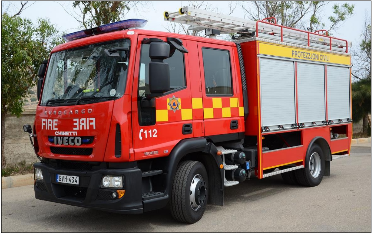
One of a pair of 2018 Iveco Eurocargo 120E25/Chinetti pumpers delivered to the Maltese Fire Service. They are equipped with 2400LPM pumps. (Photo from Anthony Pisani)
