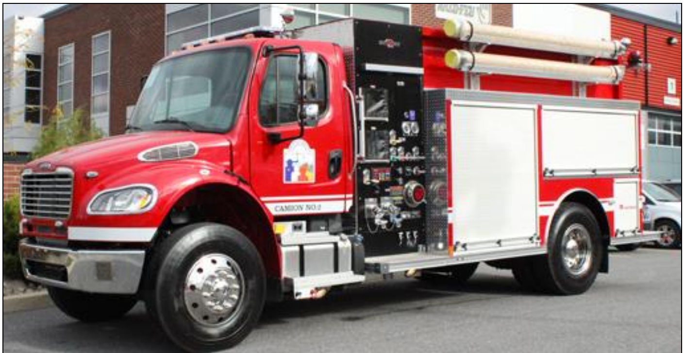
Petit-Rocher, NB No.2, a 2016 Freightliner M2-106/Rosenbauer 1050igpm Darley pump and a 1000gwt (Aerofeu photo)
