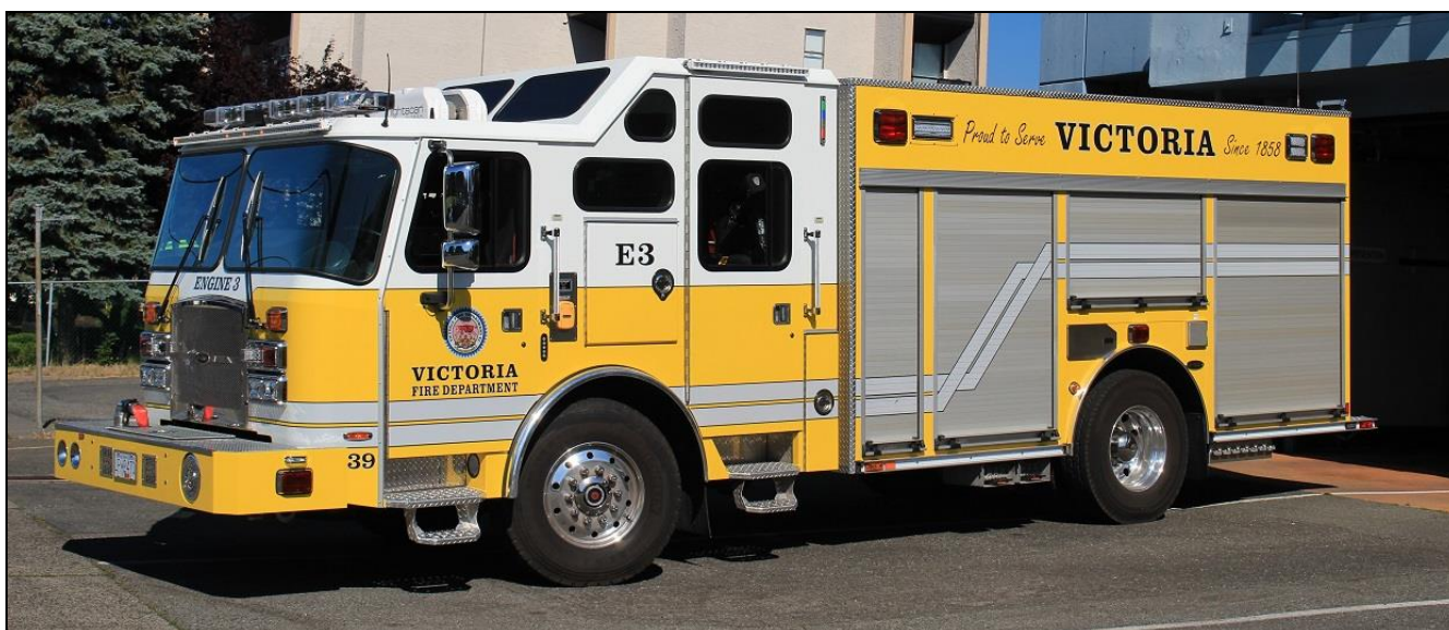
Victoria, BC Engine 3, a 2017 E-1 Typhoon, a 1250igpm/440gwt/20gft(A)/20gft(B) #141080. (Dave Stewardson photos)
