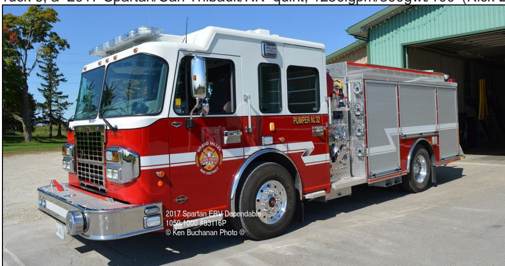
Grand Valley, ON Pumper 32 is a 2017 Spartan Gladiator/Spartan ERV/DEV rig, With a 1050igpm pump and a 1000gwt. (Ken Buchanan photo)
