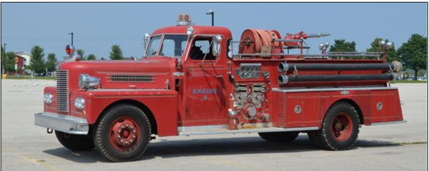
Ex Racine Engine 9, a 1963 Pirsch 1000gpm pump, 300gwt, S#2661(Bob Rupert photos)
