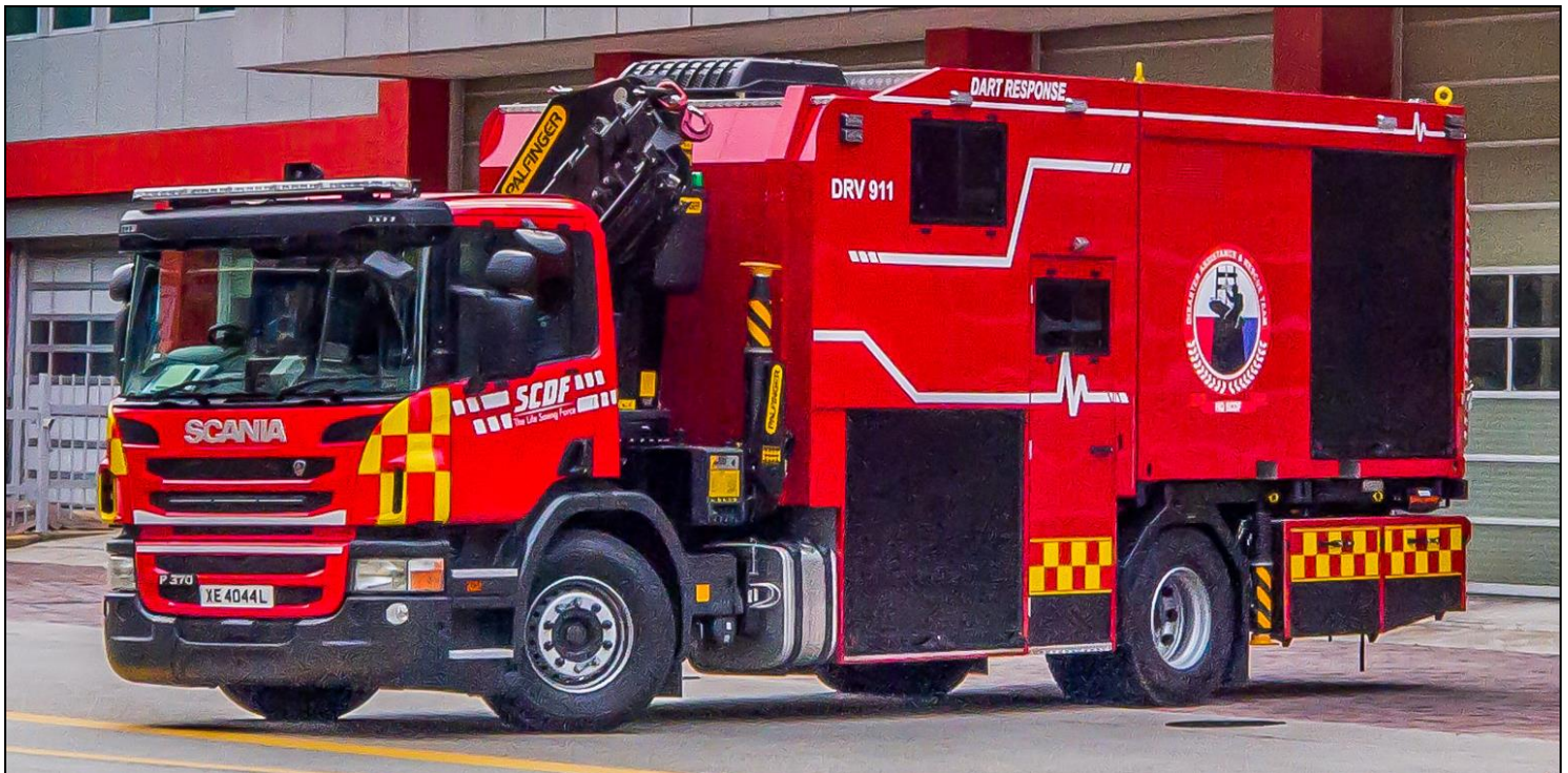
One of the two new heavy rescues from Singapore. DRV 911 was built on a 2018 Scania P370 chassis by Rosenbauer and features a Palfinger crane for lifting or stabilizing large vehicles. It is primarily for responding to incidents involving trucks and other large vehicles, structural collapses and trench rescues. The module on the back is removable. (Kenneth Lai photo)
