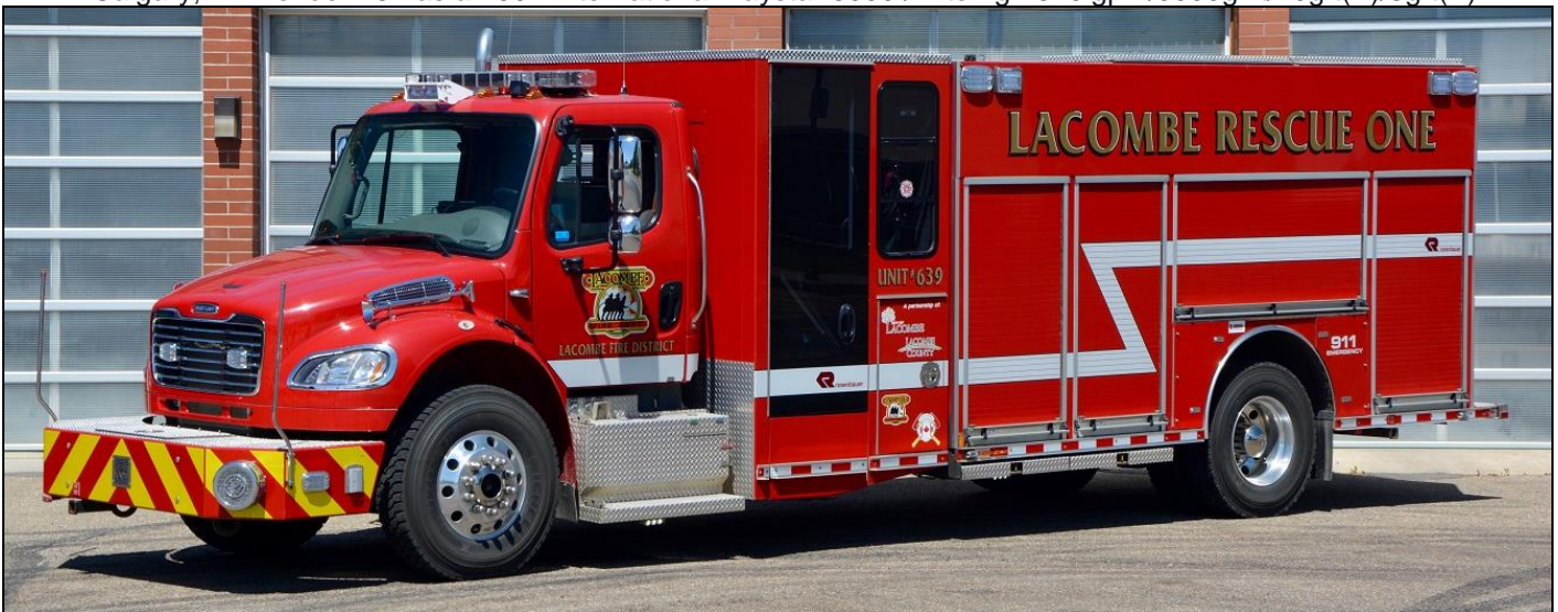
Lacombe, AB Rescue 1, a 2012 Freightliner M2-106/Rosenbauer heavy rescue.
