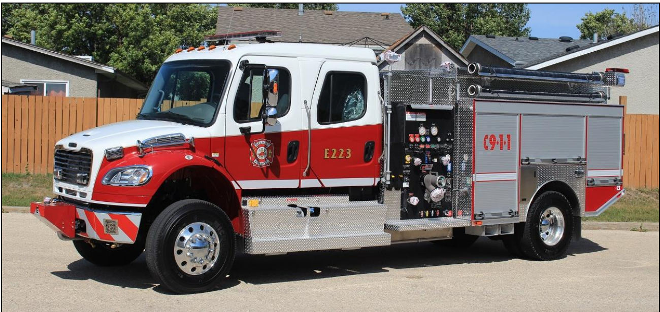
Melfort, SK Engine 223 , a 2018 Freightliner M2 106 4x4/ Fort Garry wildland pumper.
