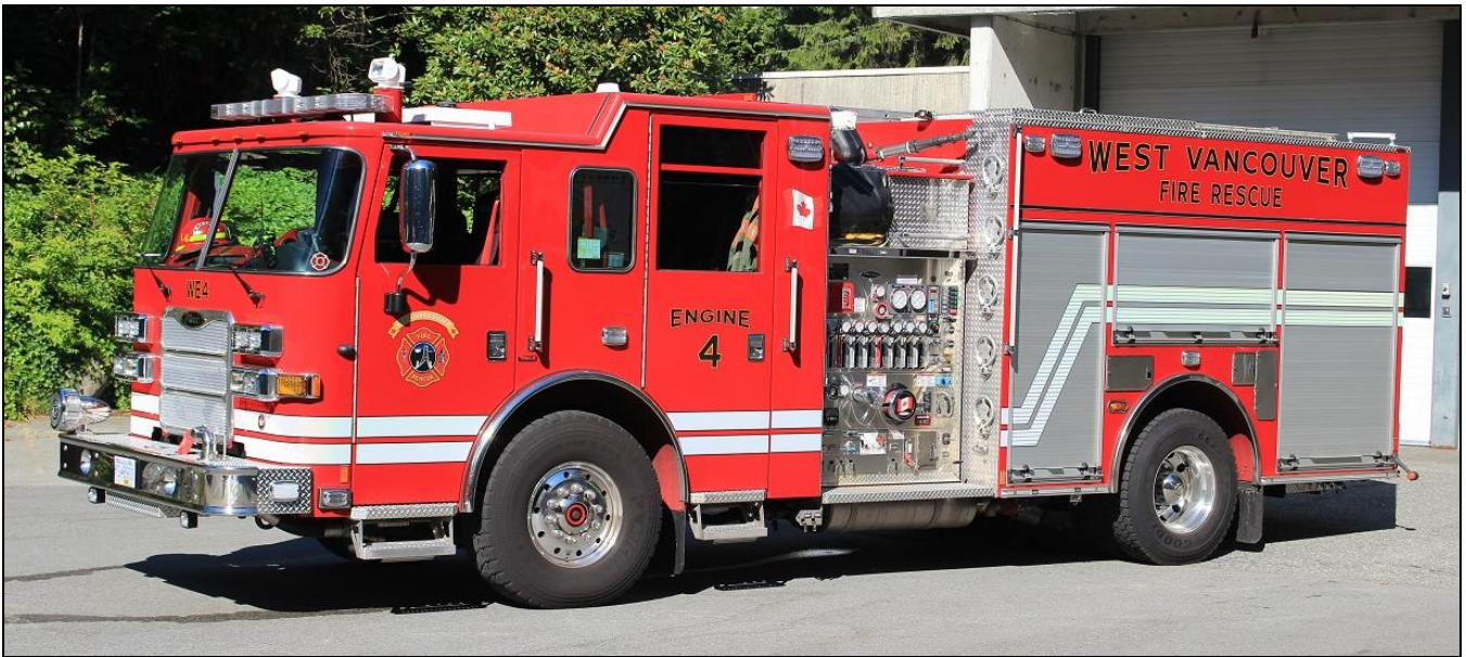
West Vancouver, BC Engine 4, 2016 Pierce Arrow XT, 1750igpm/344gwt/30gft s/n 30100
