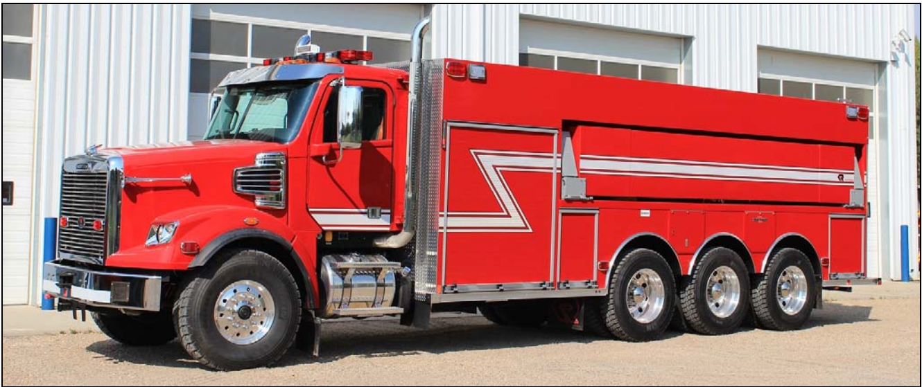
This is Rosenbauer's first four axle tanker. Just delivered to Valleyview, AB, on a Freightliner Coronado chassis, it has a 420igpm pump and a 4000gwt.
