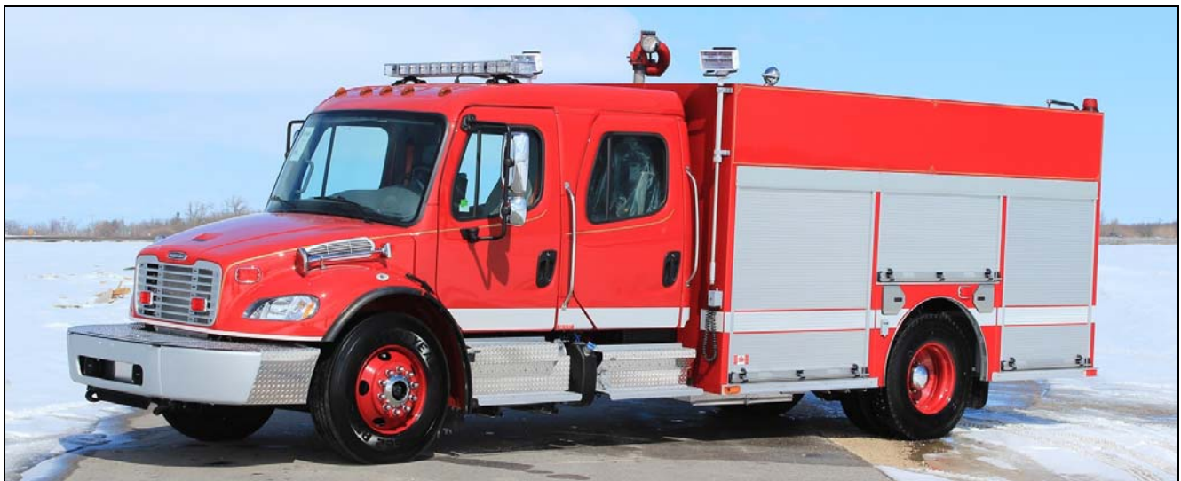
Magrath, AB got this 2014 Freightliner M2-106/Fort Garry pumper during the winter. It came with a 1050igpm pump, 800gwt and 25gft. It also has a CAFS, s/n M509. (Dave Stewardson photos)
