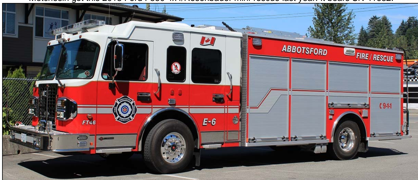
This 2014 Spartan Metro Star/Hub pumper went to Abbotsford last April. Engine 6 sports a 1500igpm Hale pump, and a 500gwt. (Dave Stewardson photos)
