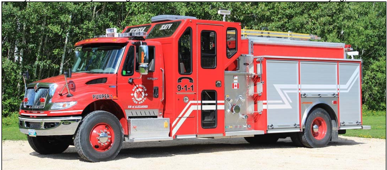
Late last year Bird River, MB put this 2013 IHC 4400/Acres pumper in service. It sports a 1050igpm pump, and an 800gwt (s/n 131220111). (Dave Stewardson photos)
