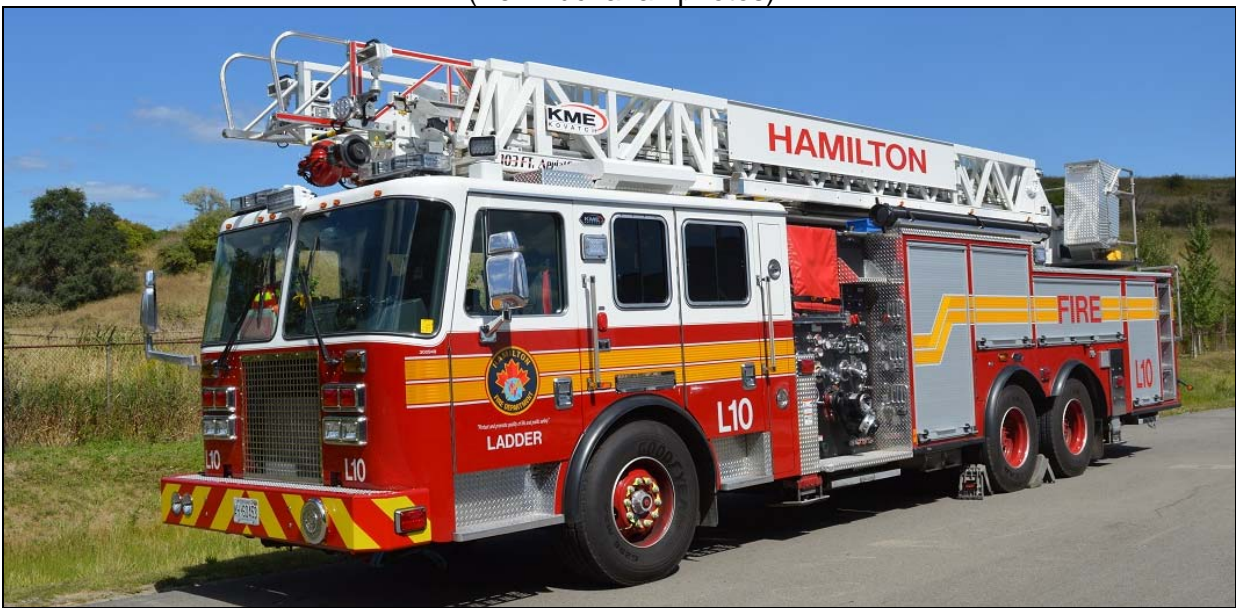
Niagara Falls P.6 2013 Freightliner M2/Spartan ERVDEV 1500gpm/1000gwt (SN 211093-1) and Hamilton's new Ladder 10, a 2014 KME Predator quint with 2000igpm/500gwt/25gft/103' (Ken Buchanan photos)
