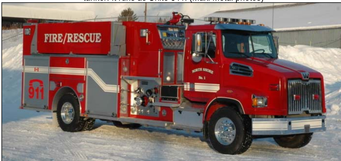
North River, PEI Unit 3 a 2017 Freightliner M2-108SD/Metalfab 1250igpm/3000gwt/50gft
