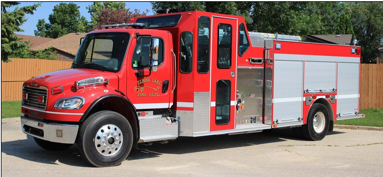
Elbow Lake, MB, a 2017 Freightliner M2 106/Fort Garry pumper 1500igpm/1000gwt/30gft (SN#M796)
