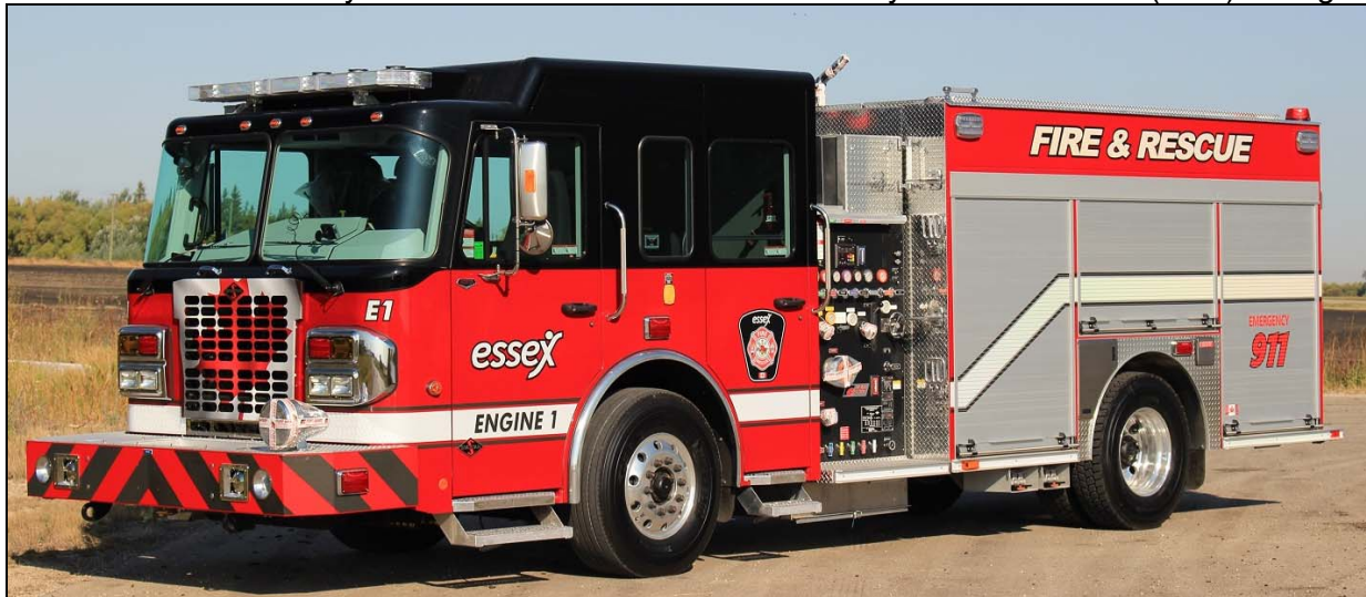
Essex Engine 1 is now running this 2017 Spartan Metro Star/ Fort Garry pumper, it has a 1050igpm pump, 800gwt and 25gft. SN M870 (Dave Stewardson photos)
