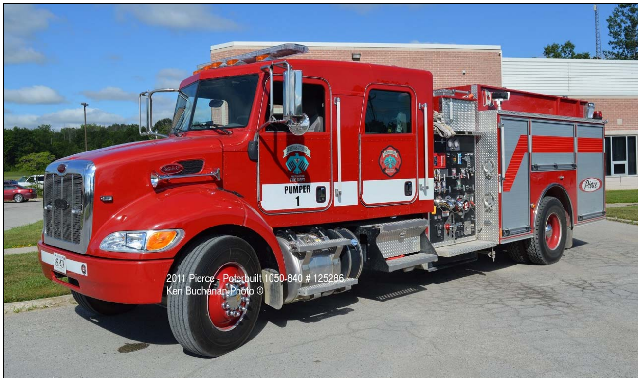
Pump 1 is a 2011 Peterbuilt Pierce pumper with a 1050igmp pump and an 844gwt. S/N 125286
