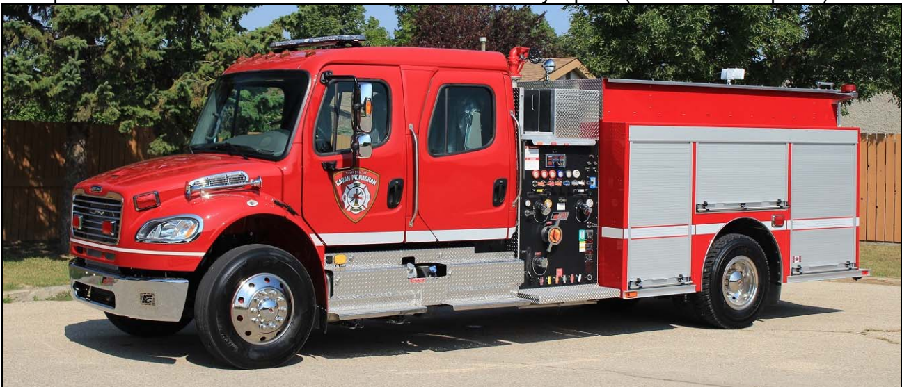
Cavan-Monaghan just got two of these 2017 Freightliner M2-106/Fort Garry rigs. They have 1050igpm Hale pumps, 800gwts and 25gfts s/n M781 above, went to Keene. (Dave Stewardson photo)
