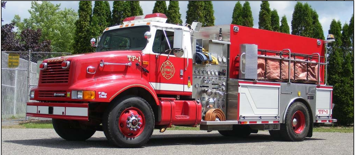
Otisco, NY TP.1 is an 1999 International/Saulsbury pumper-tanker, 1500gpm/1500gwt.
