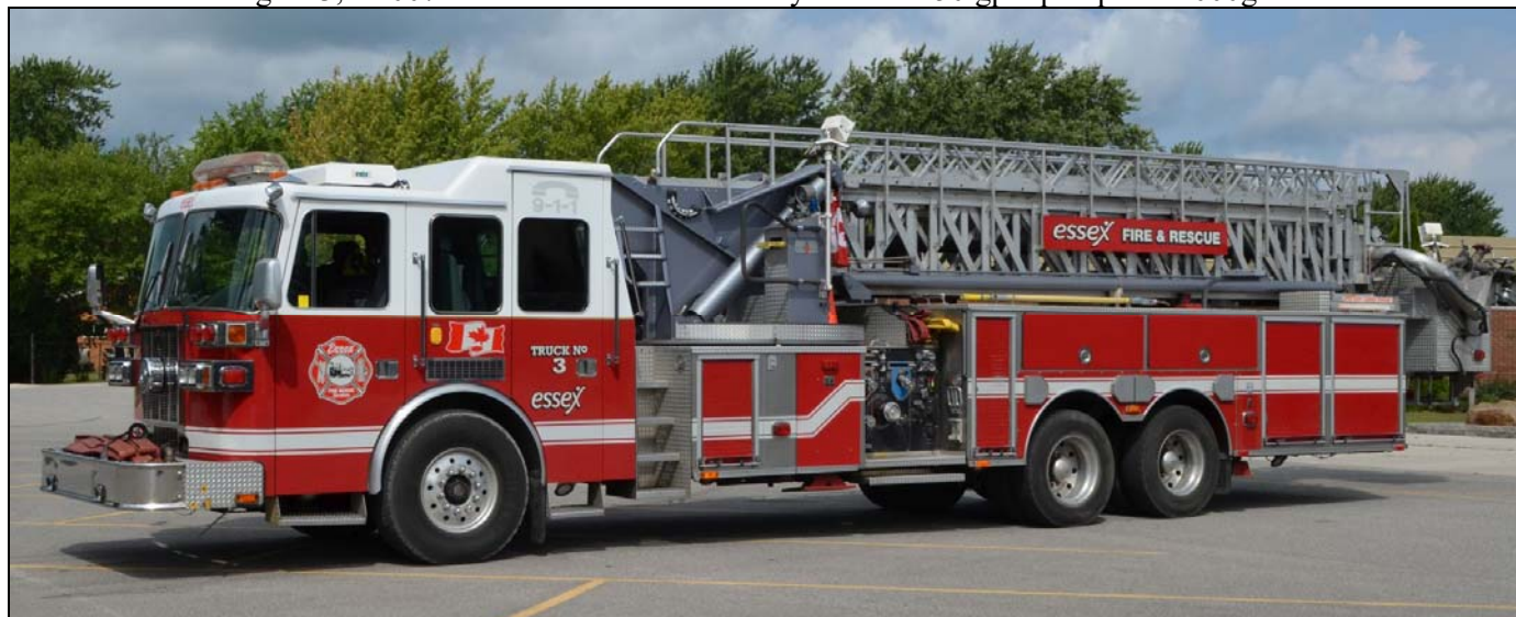
Essex Truck 3, a 1998 Sutphen 95' tower with a 1250igpm pump and 300 gwt. S# HS 3290 (Bob Rupert)
