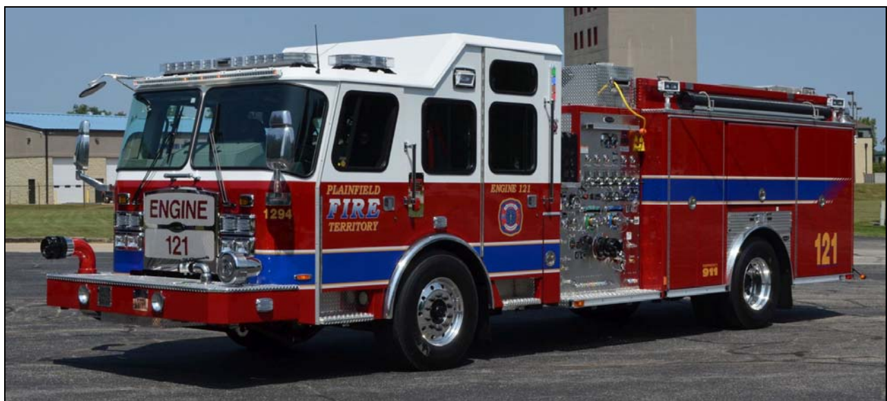
Plainfield Twp. IN Engine 121 is a 2017 E-One Cyclone pumper. 2000gpm/1000gwt SO# 141047 (Bob Rupert photos)
