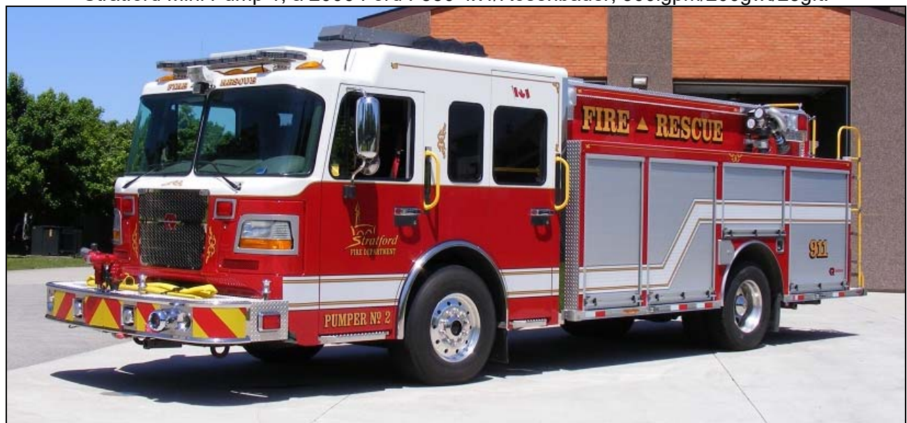
Pumper 2: 2008 Spartan MFD/Rosenbauer Commander 1050igpm/625gwt/2x20gfts. (SN 113018) (Neil McCarten photos)
