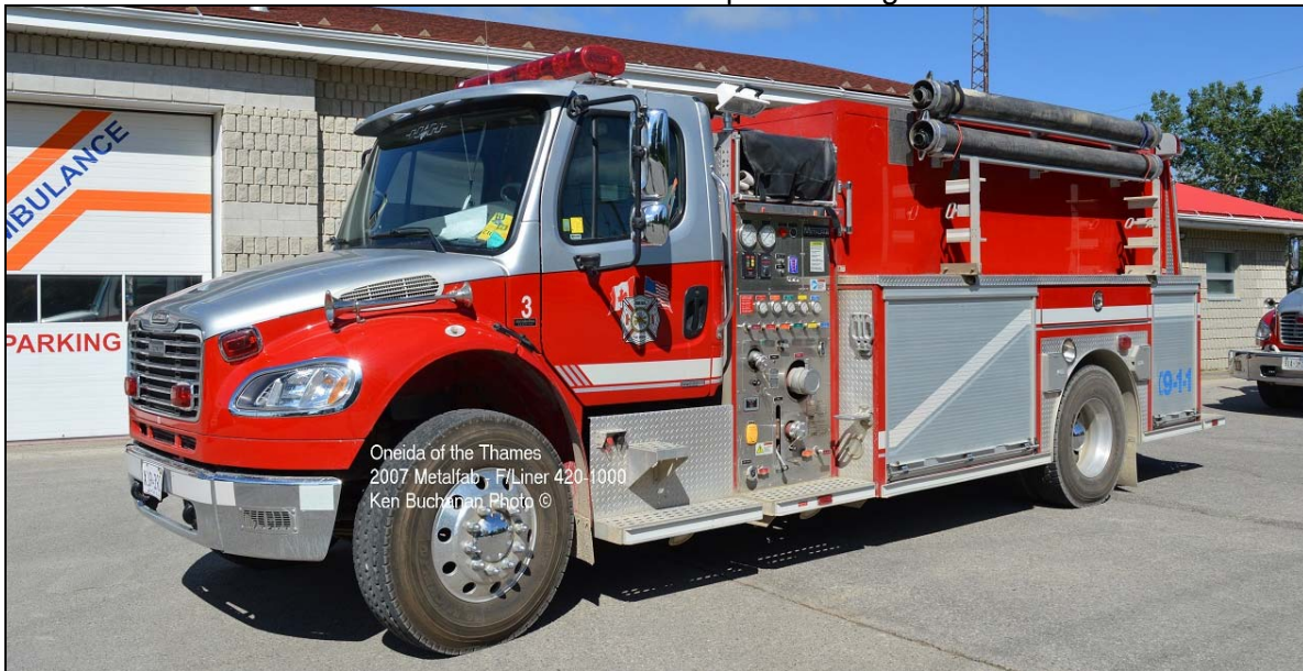
Tanker 3 2007 Freightliner M2/Metalfab 420igpm/1000gwt. (Ken Buchanan photos)
