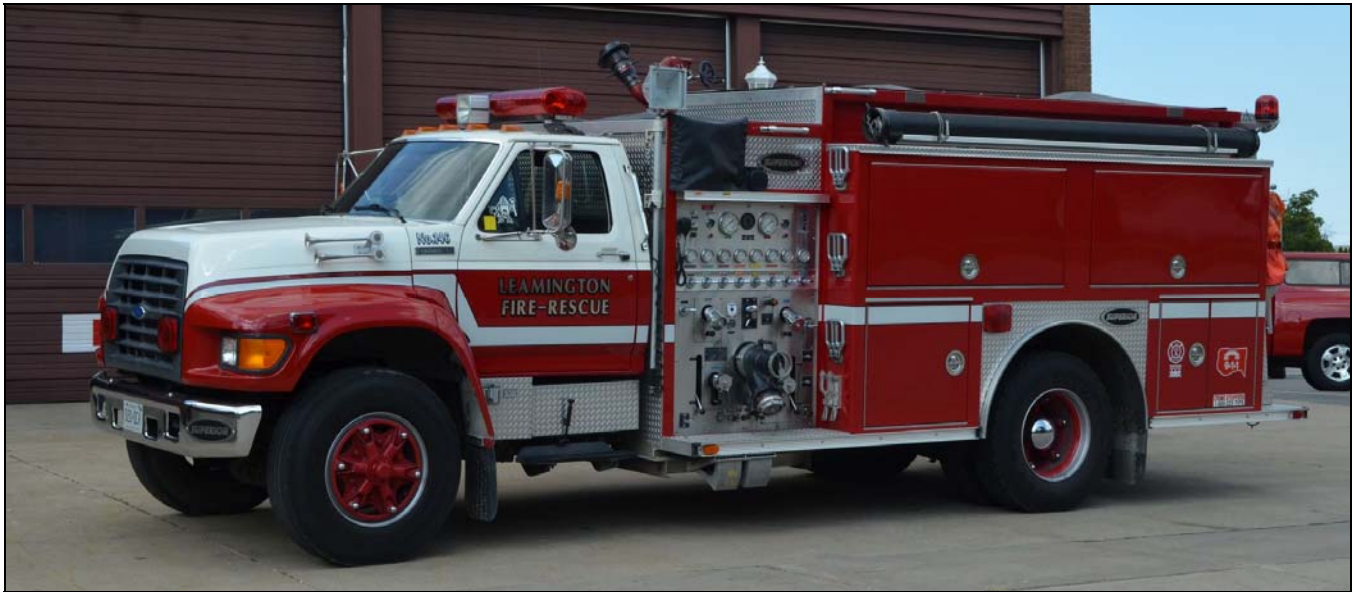
Leamington Unit 146 is a 1997 Ford F800/Superior pumper 1050igpm pump and 1000gwt. S# SE1701
