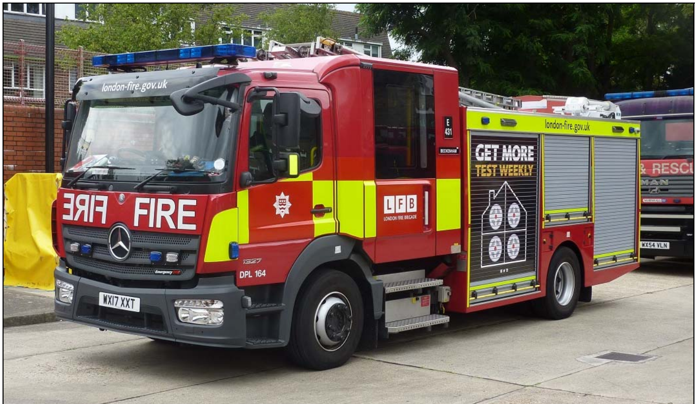
This is one of the 52 new replacement pumps being currently allocated to LFB stations, this particular one to Station E43 Beckenham in LFB South-East Area. They are supplied by Mercedes-Benz on Atego 1327F chassis with bodywork by Emergency One (UK), having 272 bhp engines, 660 gpm pumps, 300 gallon water tanks and 17 gallon foam tanks. They also have two 22mm high-pressure hose-reels, a larger diameter than fitted to previous pumps, which are said by crews to be as effective as inch-and-three-quarter hose lines. (Bill Hickin)
