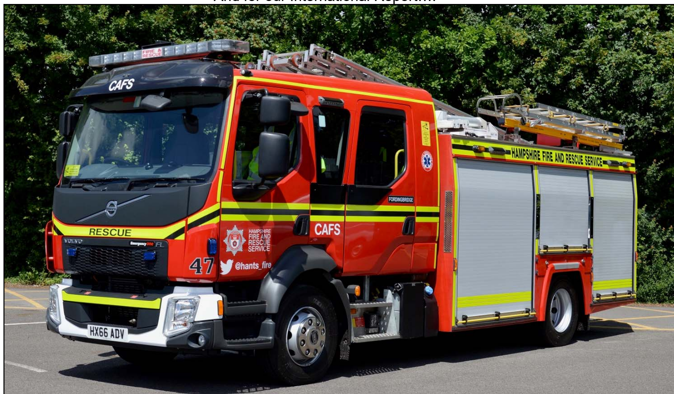
No 1 – The newest pumping appliance in Hampshire Fire and Rescue Service is this Volvo FL260 with Emergency One (UK) bodywork. HX66 ADV is allocated to the “On Call” station at Fordingbridge in the New Forest.
