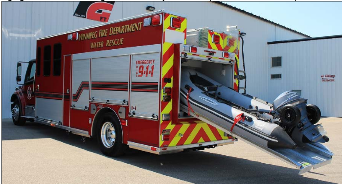
An extended look at Winnipeg's new water rescue unit, it features an interior compartment for crews to change gear and a rear storage area with a hydraulic ramp for the rescue boat. (D. Stewardson)
