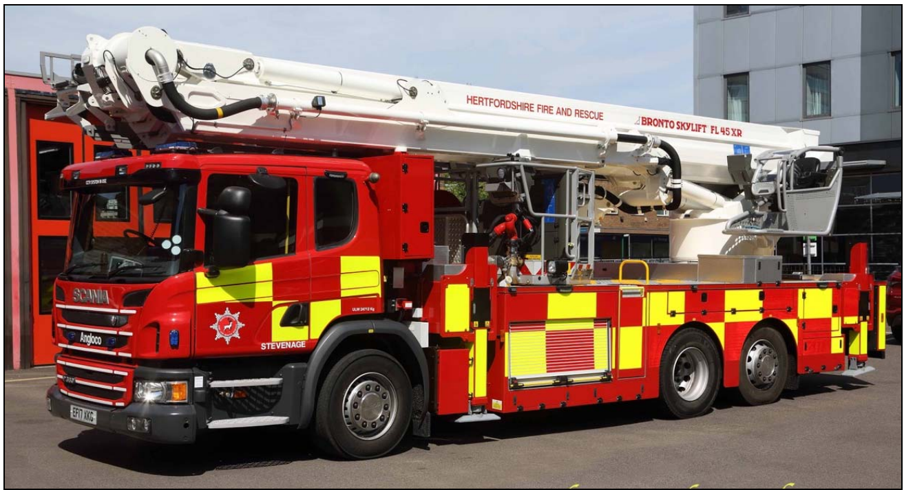
This is the U.K.s highest reach appliance. This 2017 Scania/Angloco/Bronto 45m (150') platform is now based at Stevange in Hertfordshire. (Andrew Henry photo)
