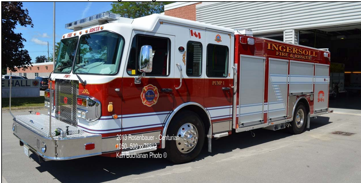
Ingersoll, Pump 1: 2013 Rosenbauer Centurian 1050igpm/500gwt xx76812
