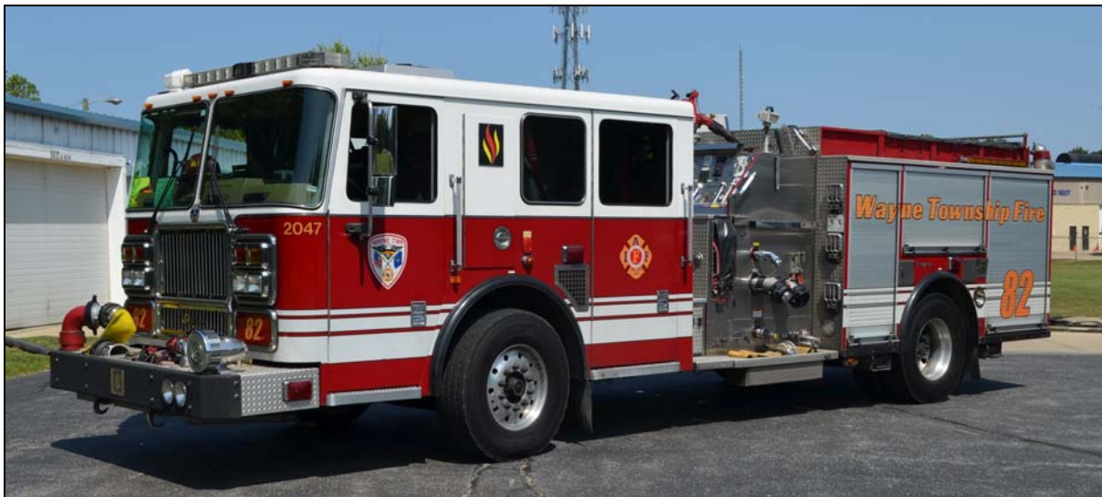
Wayne Twp, IN Engine 82, a 2007 Seagrave Marauder, 2000gpm/500gwt, S#78F58
