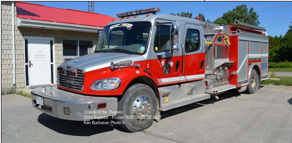
Pump 1: 2004 Freightliner M2/Superior, 1050igpm/1500gwt. SE-3237
