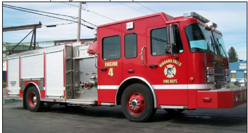
Engine 4, a 2011 Spartan Gladiator/Rosenbauer 1500gpm/750gwt/30gft (Empire Fire photo)
