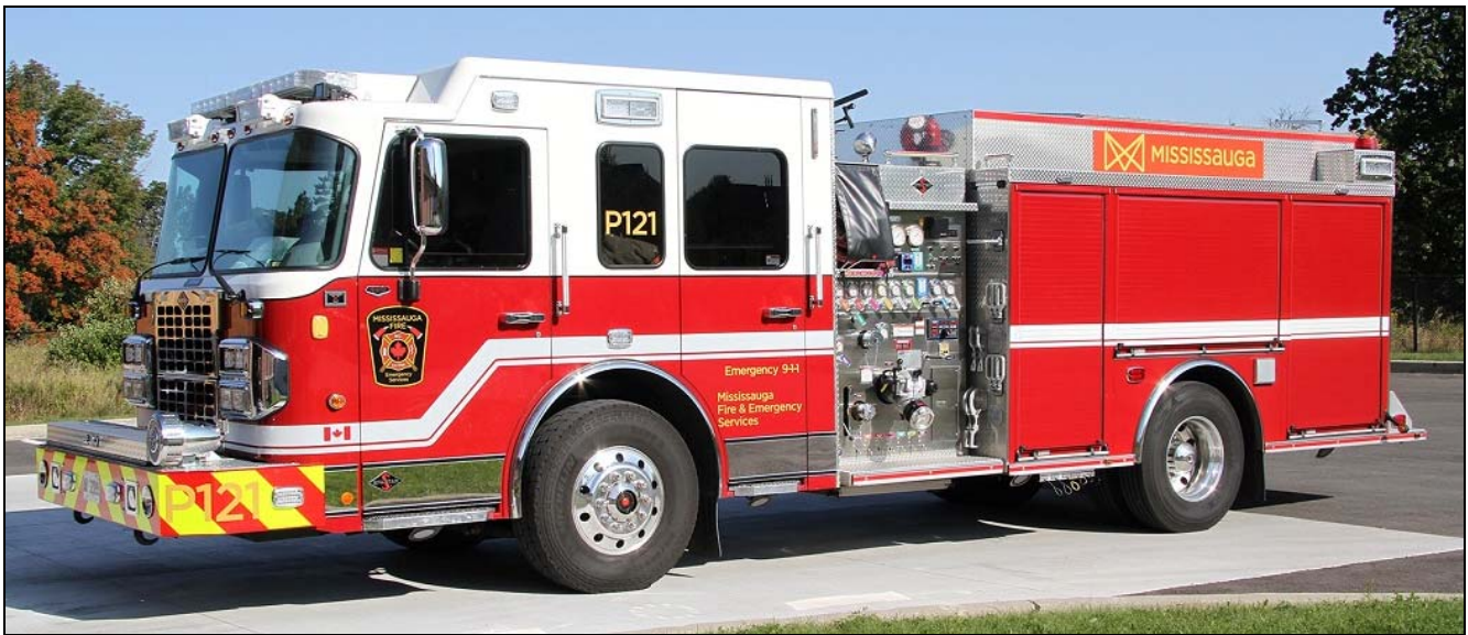
Mississauga received this 2016 Spartan Metro Star/ERV/DEV collaboration last year. It has a 1500gpm Waterous pum and a 1000gwt. S/N 216016 (Ian Duke photo)
