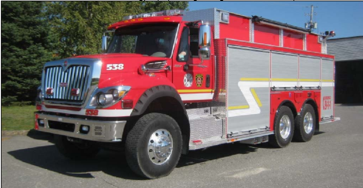
East Broughton Unité.538 2017 IHC Workstar/ Maxi Métal tanker, 3000gwt (MMFT)
