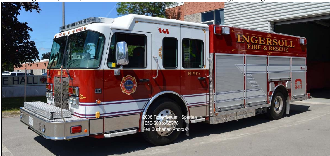
Pump 2: 2008 Spartan/Rosenbauer 1050igpm/600gwt xx65778
