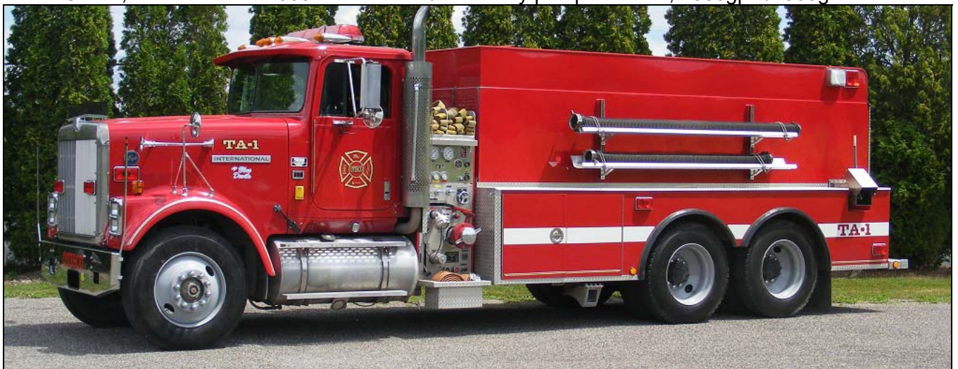
Otisco, NY TA.1 is a 1984 International Transtar tanker, 500gpm/2500gwt. (Ken Walton photos)
