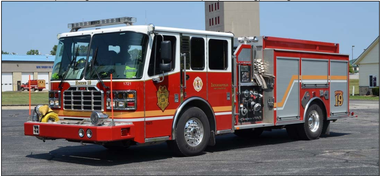
Indianapolis Engine 19, a 2011 Ferrara Inferno pumper, 2000gpm/500gwt, S# H4856
