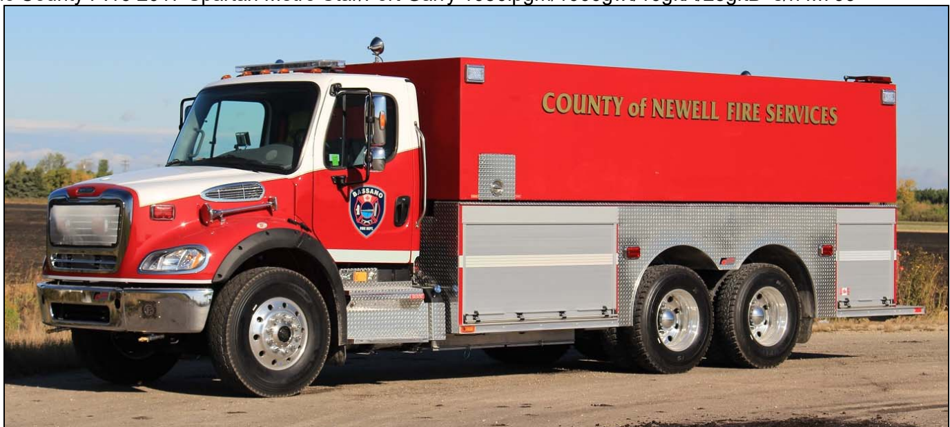
Newell County, AB received two of these 2017 Freightliner M2-112/Fort Garry tankers, they have 625igpm Hale pumps and 3000gwts S/N M842, above, went to Bassano, S/N 841 to Rolling Hills.
