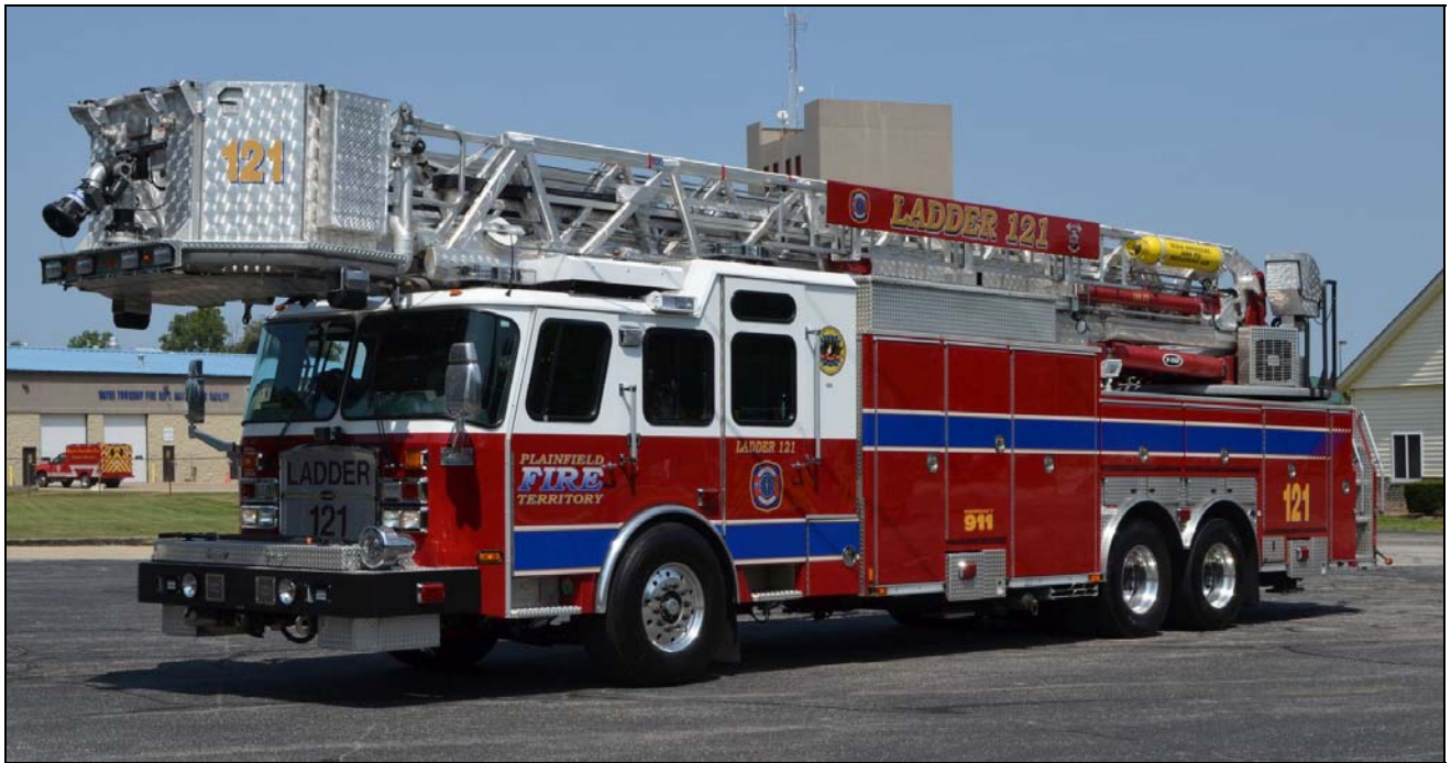
Plainfield Twp. IN Ladder 121, a 2012 E-One Cyclone 100' tower, SO#137535 (Bob Rupert photo)
