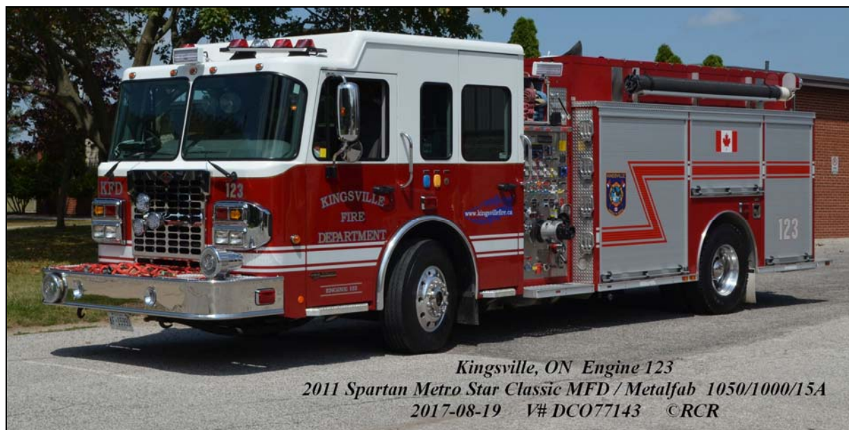
Engine 123, a 2013 Spartan Metro Star Classic/Metalfab 1050igpm/1000gwt/15gft V#DC077143
