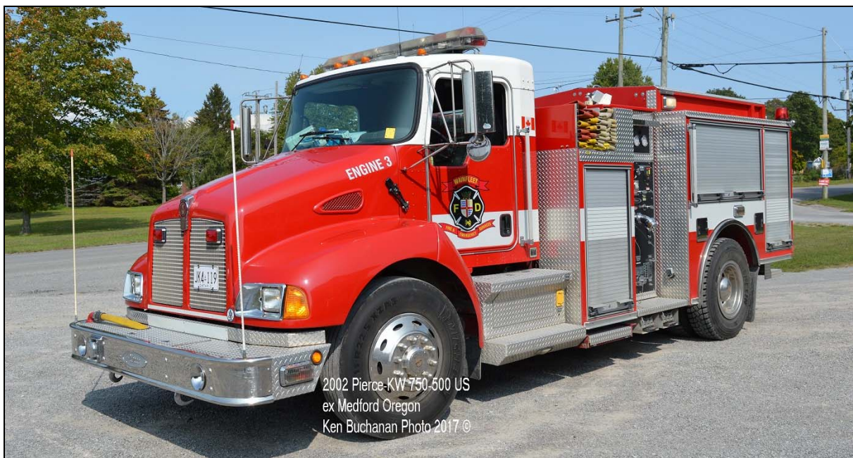
Wainfleet Engine 3 (Burnaby Station) received this 2002 Pierce-Kenworth rig three years ago. It has a 750gpm pump and 500gwt. US Job # 13487. Ex-Medford Oregon. (Ken Buchanan)
