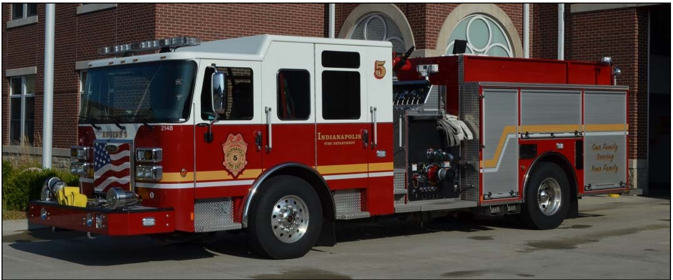
Indianapolis Engine 5, is a 2015 Pierce Saber pumper, 1500gpm/500gwt, J# 28205TR-01
