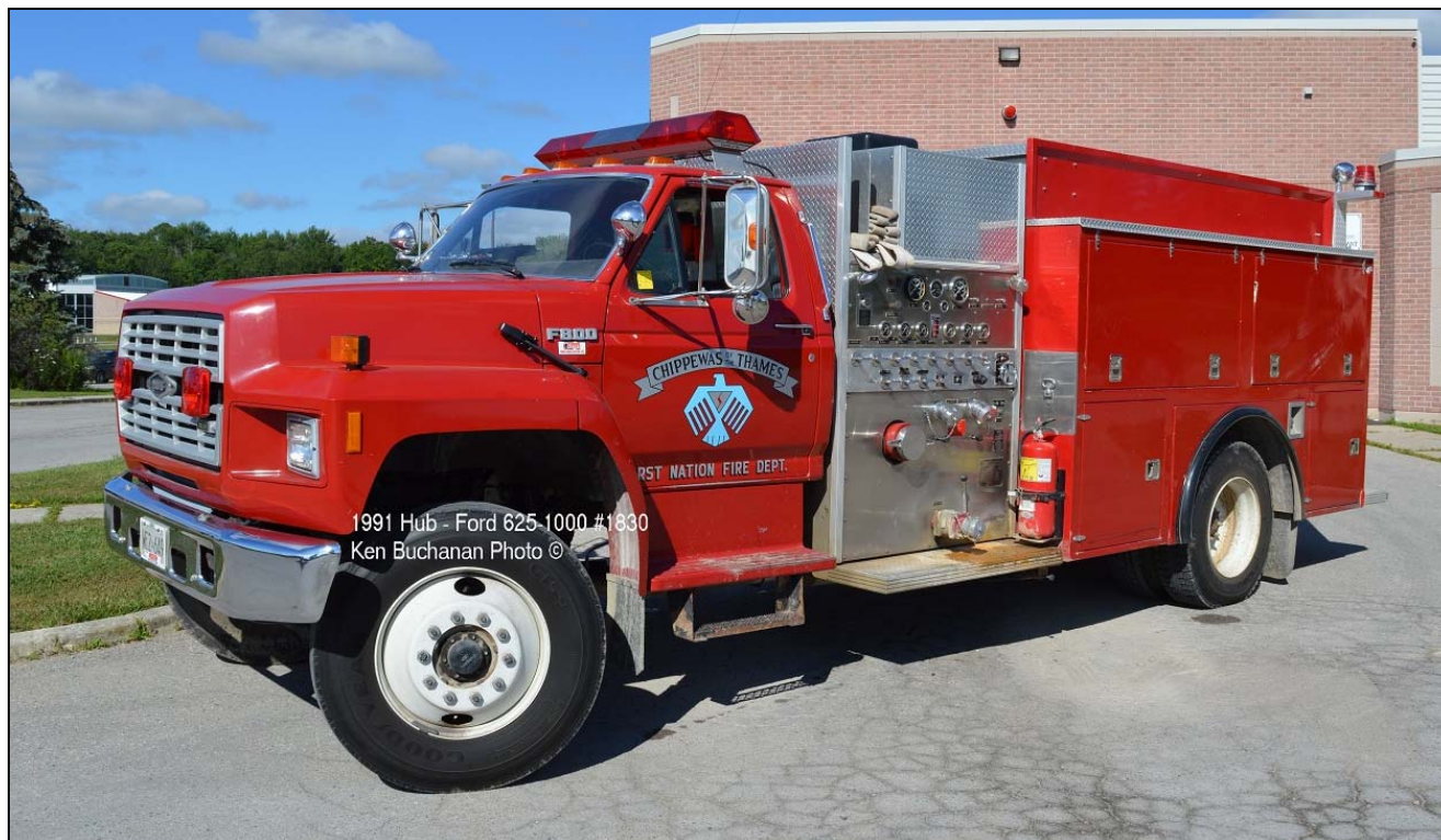
Pump 2 1991 Ford/Hub – 625igpm pump amd a 1000gwt. (Ken Buchanan photos)
