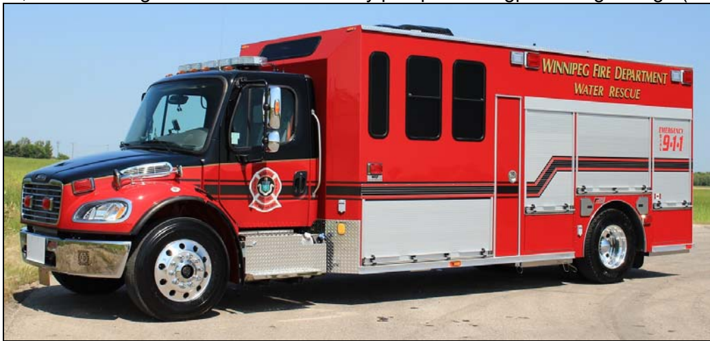
An extended look at Winnipeg's new water rescue unit, it features an interior compartment for crews to change gear and a rear storage area with a hydraulic ramp for the rescue boat. (D. Stewardson)
